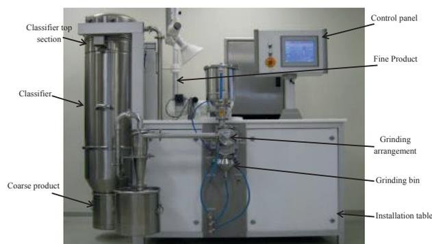
Fig. 1 Alpine Turboplex - Ultrafine Classifier 50 ATP, prepared in collaboration with [26]
