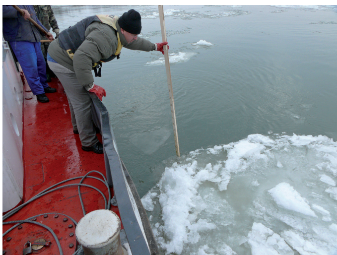
Fig. 14 Measuring ice thickness above (a) and below (b) water level on the Danube
