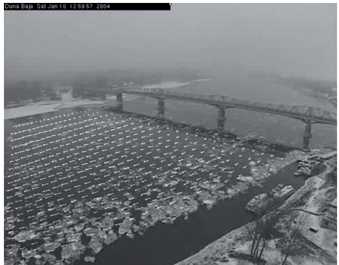
Fig. 4 PIV-reconstructed surface velocity vector field by Marian Muste, U. of Iowa
