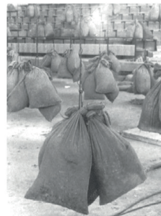
Fig. 6 In situ test of Sports Hall double layer with L = 60 m and B = 50 m.
