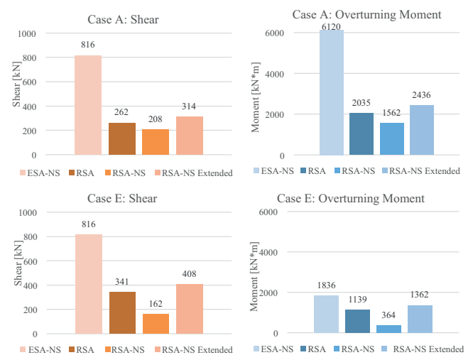
Fig. 21 Code Spectra, Case A and Case E shear and overturning moment comparison
