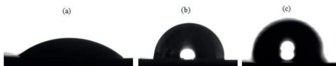
Fig. 2 The contact angles of some clay-nanocomposite composite samples. a) Contact angle image of the natural clay (37°); b) Contact angle image of the HOC (88°); c) Contact angle image of the CNCR10 sample (106.3°)
