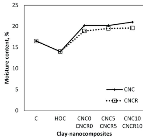
**Fig. 7** The moisture values of the clay-nanocomposites
