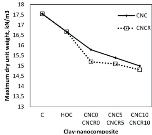
**Fig. 6** The maximum dry unit weight values of the clay-nanocomposites (compaction effort is 2597 kJ/m³)
