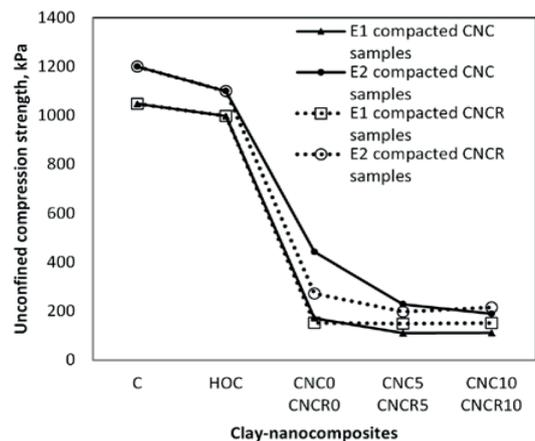
Fig. 10 The unconfined compressive strengths of the clay-nanocomposites
