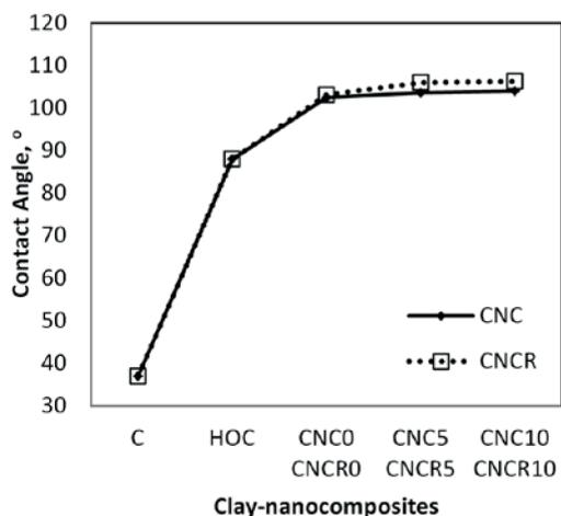
Fig. 1 Contact angle measurements of the clay-nanocomposite samples
