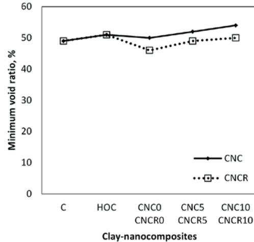
**Fig. 8** The minimum void ratios of the clay-nanocomposite samples
