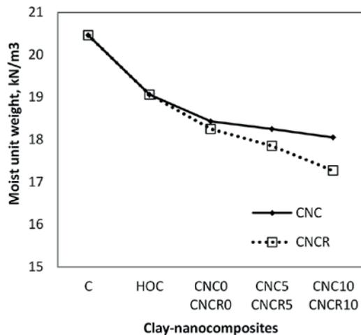
Fig. 9 The moist unit weights of the clay-nanocomposite samples
