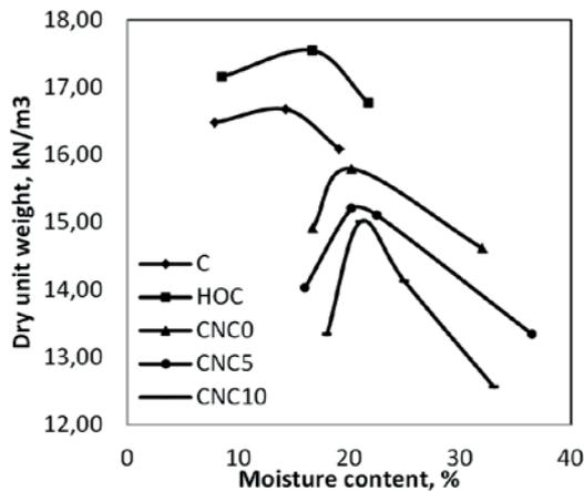
**Fig. 5** Compaction curves of the clay-nanocomposite samples
