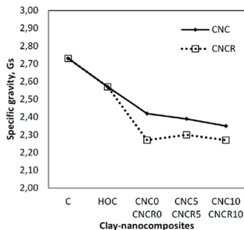
Fig. 3 Specific gravities of the nanoclay-composites
