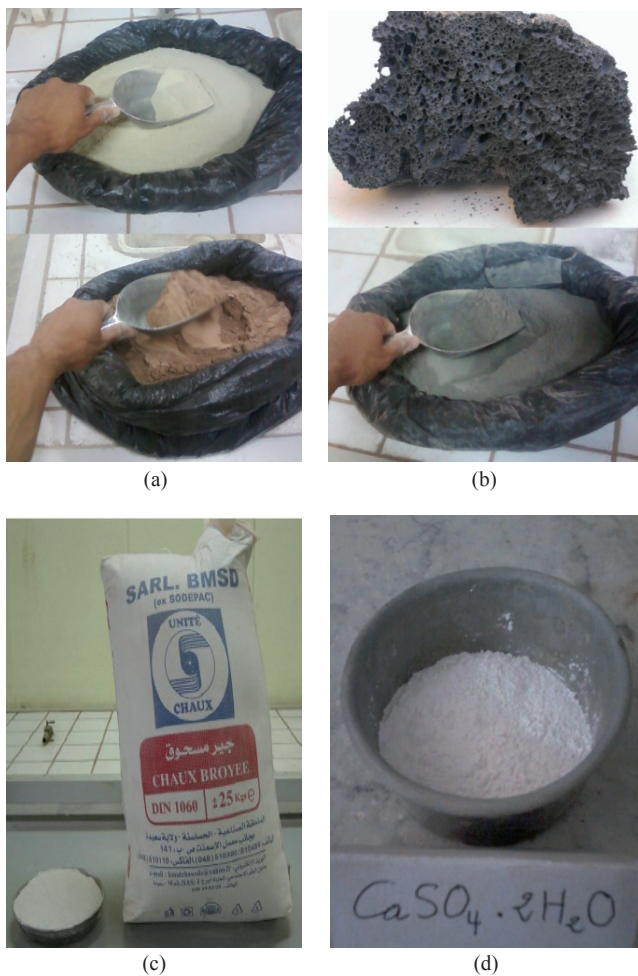
Fig. 1 Materials used and their preparation; (a) clayey soils passed to 1mm sieve, (b) NP before and after preparation, (c) hydrated lime usually used for construction purposes and (d) calcium sulphate
