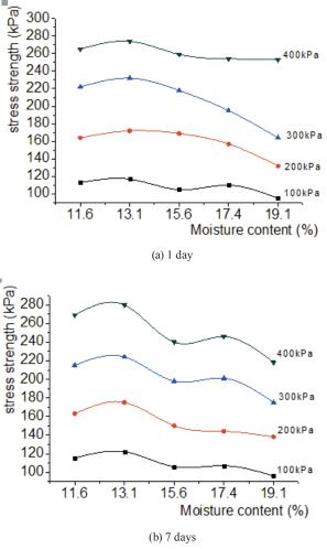
Fig. 5 Moisture content ~ shear strength curve for sample of G20
