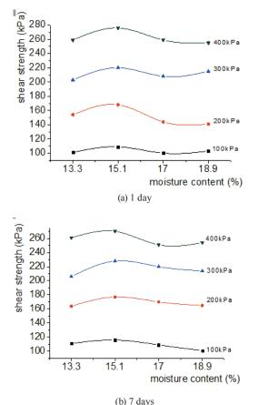
**Fig. 6** Moisture content ~ shear strength curve for sample of G30
