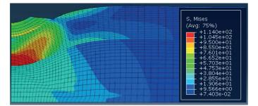
(b) Stress contours of the soil with embankment Fig. 12 Stress distribution contours after loading
