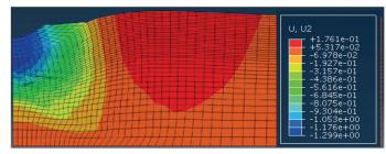
(a) The vertical settlement contours of the soil without embankment
