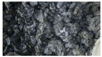
Fig. 1 EAFO steel slag before grinding and sieving
