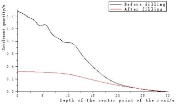
Fig. 14 Vertical settlement along the center line of the embankment
