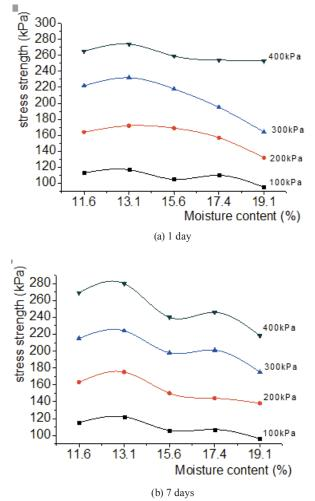
Fig. 4 Moisture content ~ shear strength curve for sample of G10
