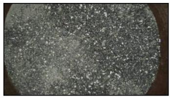
Fig. 2 EAFO steel slag after grinding and sieving
