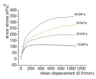
Fig. 3 Shear stress-shear displacement curve (14% moisture content of the G20 group for 1 day curing time)
