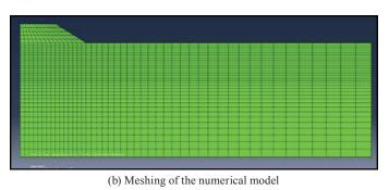
Fig. 11 Mesh partitions and the initial boundary conditions (before loading)
