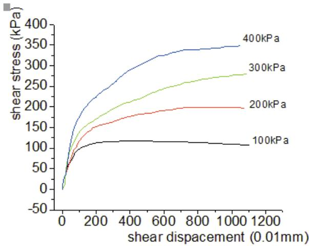
Fig. 3 Shear stress-shear displacement curve (14% moisture content of the G20 group for 1 day curing time)
