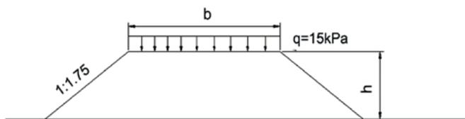
Fig. 10 Schematic diagram of embankment
