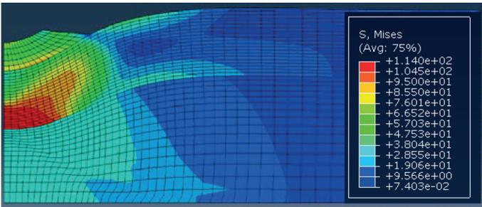
(b) Stress contours of the soil with embankment
