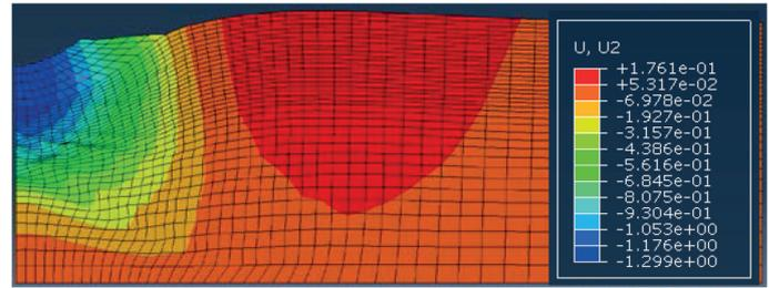
(a) The vertical settlement contours of the soil without embankment
