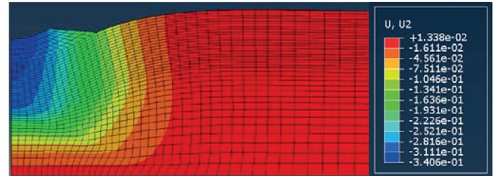
(b) The vertical settlement contours of the soil with embankment
