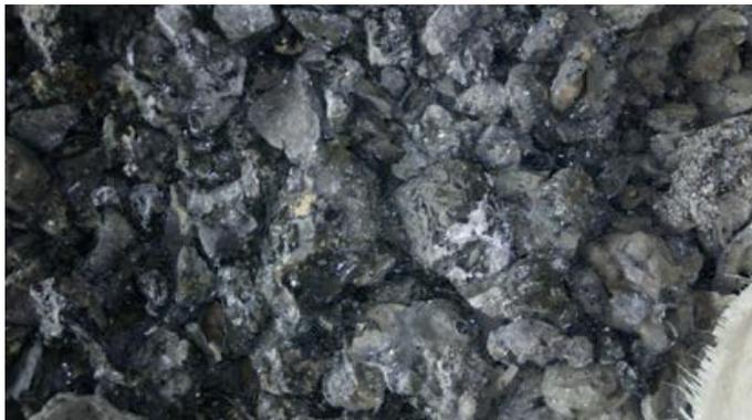
Fig. 1 EAFO steel slag before grinding and sieving
