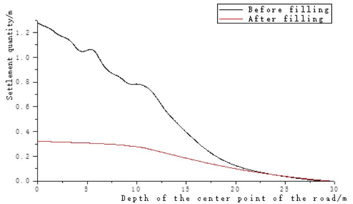
**Fig. 14** Vertical settlement along the center line of the embankment
