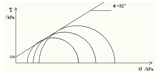
Fig. 9 Mohr circle and shear strength envelope
