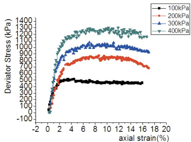
Fig. 8 Curve of deviator stress  $\sigma_1 - \sigma_3 \sim$  axial strain  $\epsilon_1$
