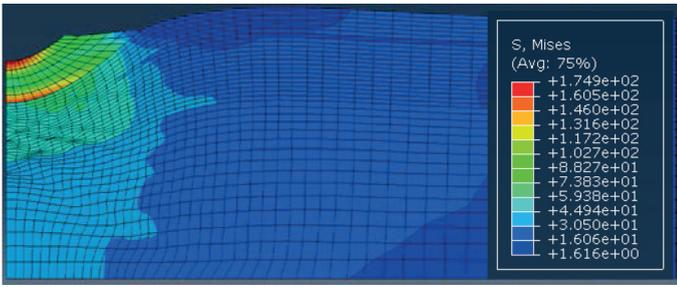
(a) Stress contours of the soil without embankment
