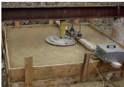
Fig. 7 Field Test Set-up for D = 30, 45, 60, 90 cm (Laman et al. [17])
