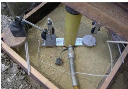
Fig. 8 Field Test Set-up for D = 6, 9, 12 cm (Laman et al. [17])
