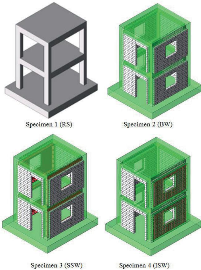
Fig. 4 3D view of specimens
