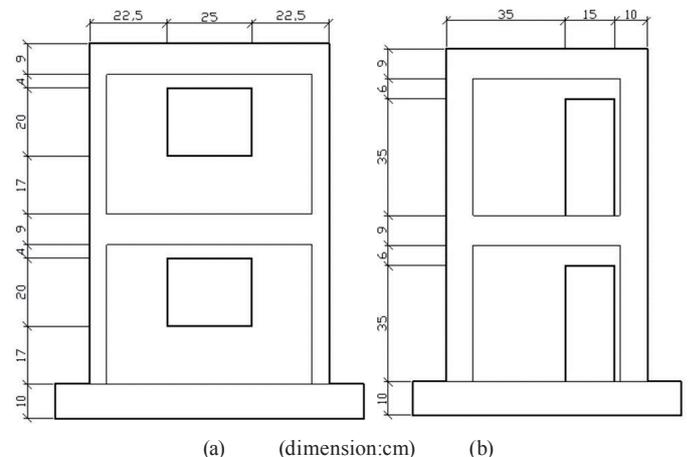
Fig. 3 Dimensions of window and door openings
