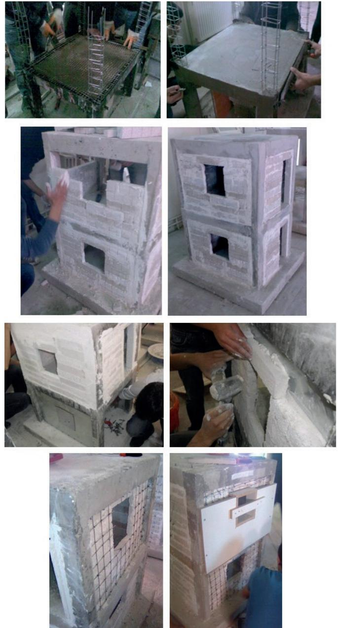
Fig. 5 Production stages of samples
