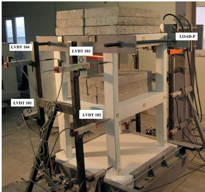
Fig. 6 LVDTs location points for displacement measurement
