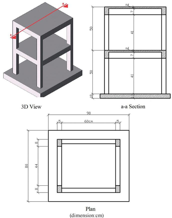
Fig. 2 Dimensions of the general specimen
