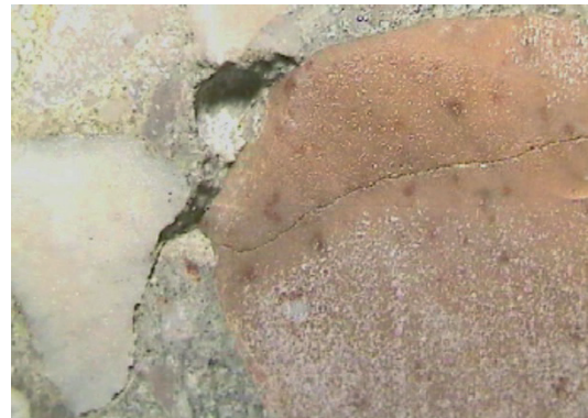
Fig. 18 Cracks around the perimeter of aggregates and inside the reddish aggregate (sample label: Beam 3).
