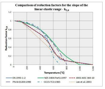
Fig. 2 Reduction factors for the slope of the linear elastic range (relative to  $E_{u}$ ) - comparison
