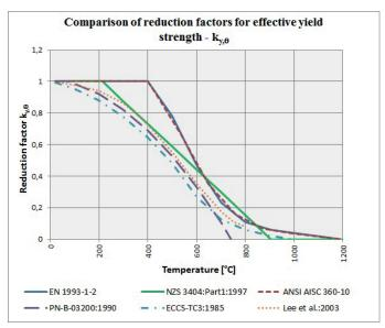
Fig. 1 Reduction factors for effective yield strength (relative to  $f_v$ ) - comparison
