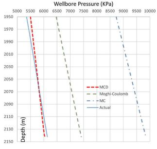
Fig. 11 Minimum mud weight prediction according damage theory and comparison with other criteria
