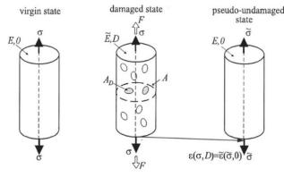
Fig. 7 a sample under damage [22]
