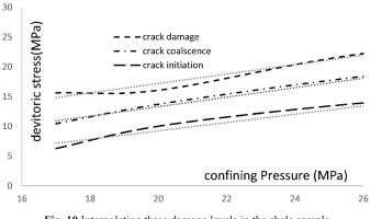
Fig. 10 Interpolating three damage levels in the shale sample
