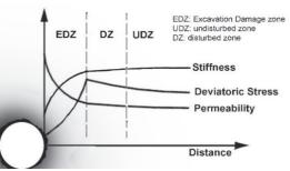
Fig. 5 Hydro mechanical changes around an excavation
