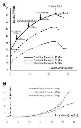
Fig. 8 (a) Stress-strain curve for shale under different confining stress,(b) Volumetric strain – axial strain curve
