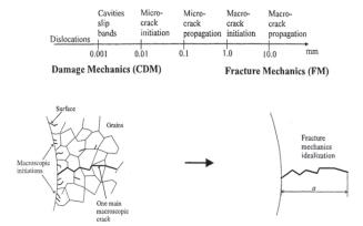
Fig. 6 The area of fracture and damage mechanics study [22]
