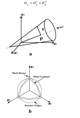
Fig. 3 a) typical yield surface, b) rock failure criterion view from hydrostatic line
