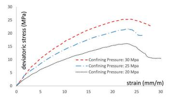
Fig. 9 deviatory stress -strain curve
