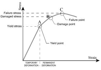
Fig. 2 Stress-strain diagram
