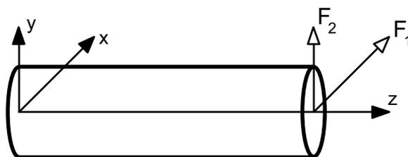
*Fig. 1.* Robot leg: a piezoceramics cylinder
