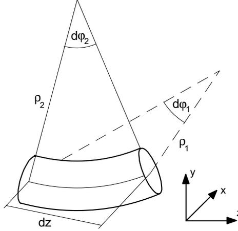
Fig. 2. Mechanical bend: part of the piezo cylinder
