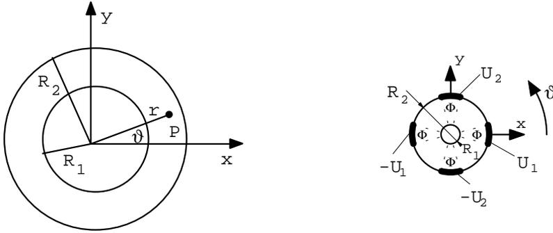
Fig. 3. Cross-section of a tubular type piezo leg
