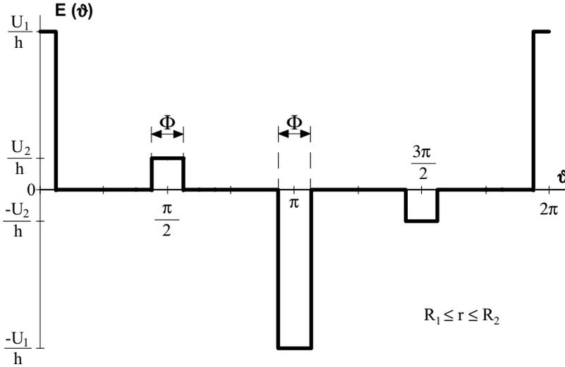
Fig. 4. Distribution of the electric field in the piezo tube
