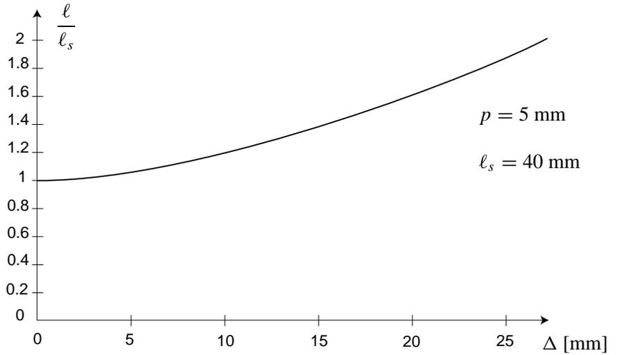
Fig. 3. Equivalent excitation length vs. the air gap
