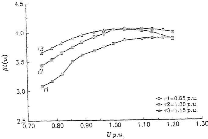
Fig. 6.  $\beta_i(u)$  of the measured pure inductive loads
