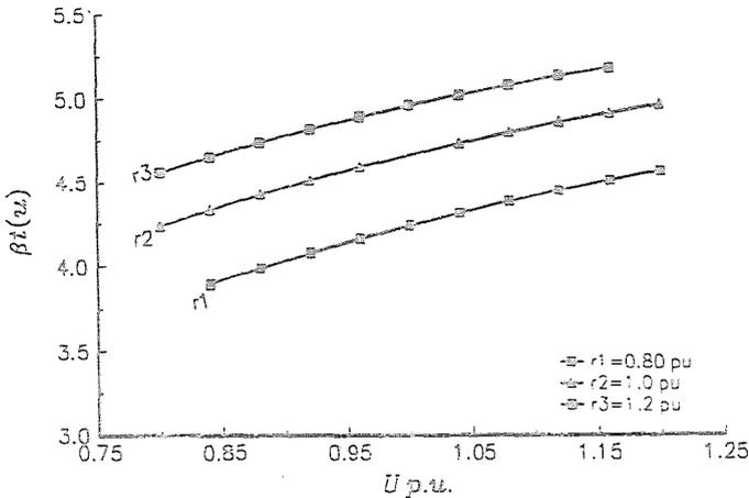
Fig. 2.  $\beta_i(u)$  characteristics of greater load with greater exponent
