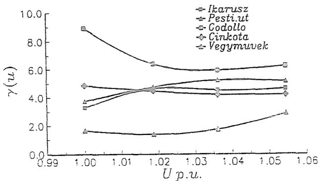
Fig. 10.  $\gamma(u)$  ranges of the measured loads
