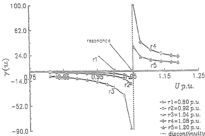
Fig. 5.  $\gamma(u)$  of the combined load, case 2 (undercompensation)
