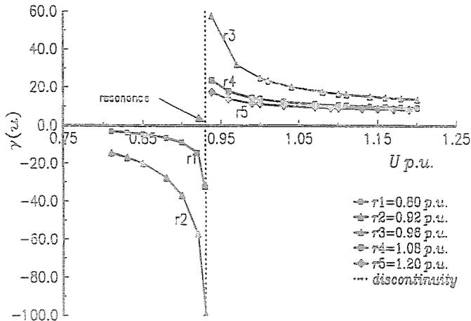
Fig. 4.  $\gamma(u)$  of the combined load, case 1 (undercompensation)
