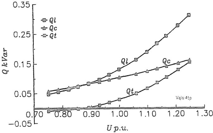
Fig. 7. Measured reactive power
