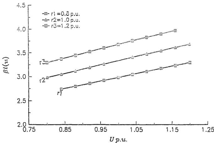
Fig. 1.  $\beta_t(u)$  characteristics of smaller load with greater exponent
