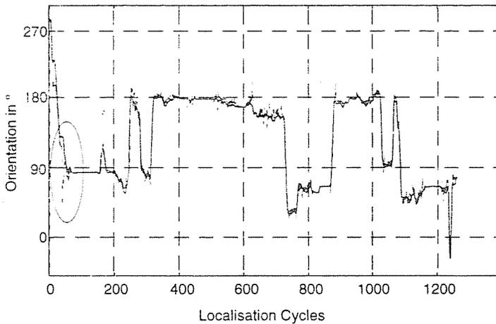
Fig. 10. Kalman filter and compass orientation for test drive
