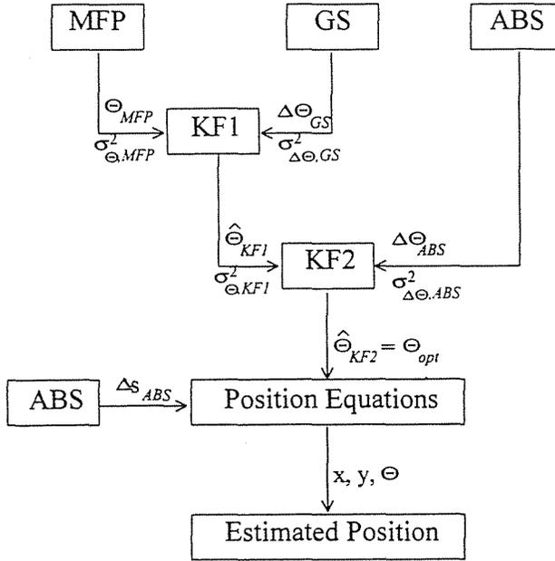
Fig. 7. Signal Flow for Data Fusion
