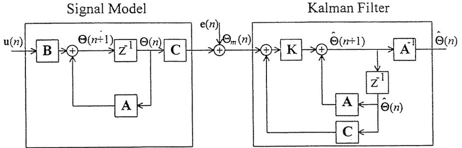
Fig. 6. Signal Model and Kalman Filter Structure
