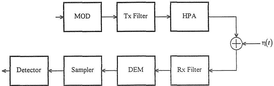
Fig. 1b. Block diagram of the system under the separated effect of HPA
