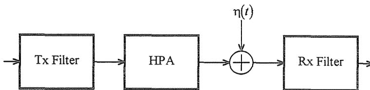
Fig. 4a. HPA is sandwiched between two filters
