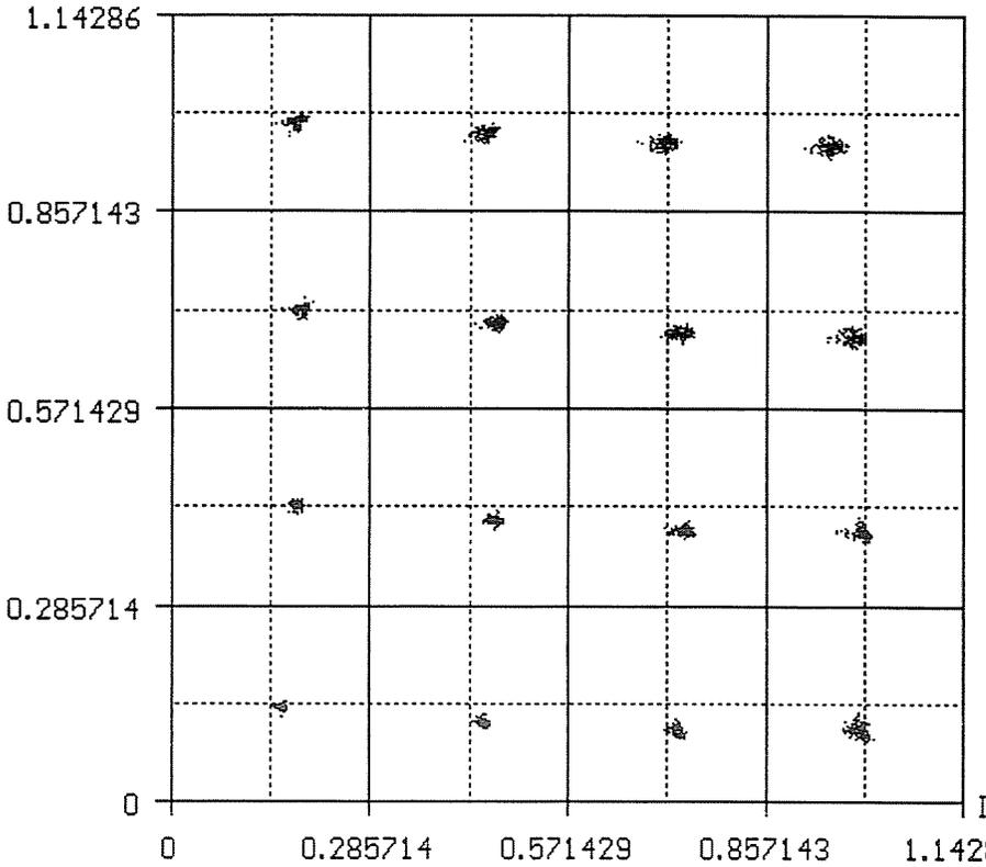
*Fig. 2.* A quadrant of 64-QAM constellation (HPA given in [4],  $BO_p = 3.5$  dB;  $\alpha = 0.5$ )
