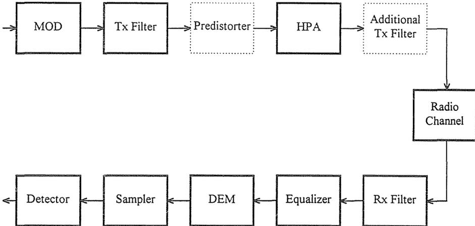
*Fig. 1a.* The model of M-QAM radio link
