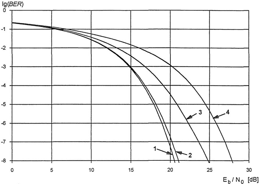
Fig. 6. Comparison of two models. 1: 1st model ( $OAPS = 0.4$  deg.), 2: 2nd model ( $OAPS = 0.7$  deg.) (HPA given in [12] with predistorter,  $BO_p = 2$  dB); 3: 1st model ( $OAPS = 2.8$  deg.), 4: 2nd model ( $OAPS = 5.3$  deg) (HPA given in [4] without predistorter,  $BO_p = 3.5$  dB)
