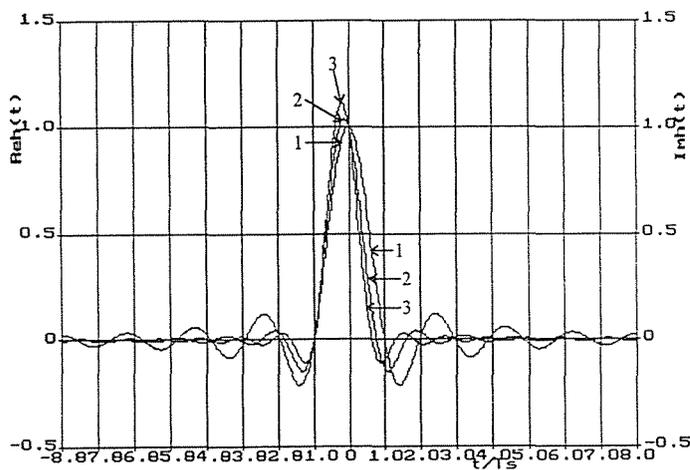
*Fig. 5.* Impulse response of the signal at the output of the  $T_x$  filter. 1:  $\alpha = 0.1$ ; 2:  $\alpha = 0.5$ ; 3:  $\alpha = 0.75$
