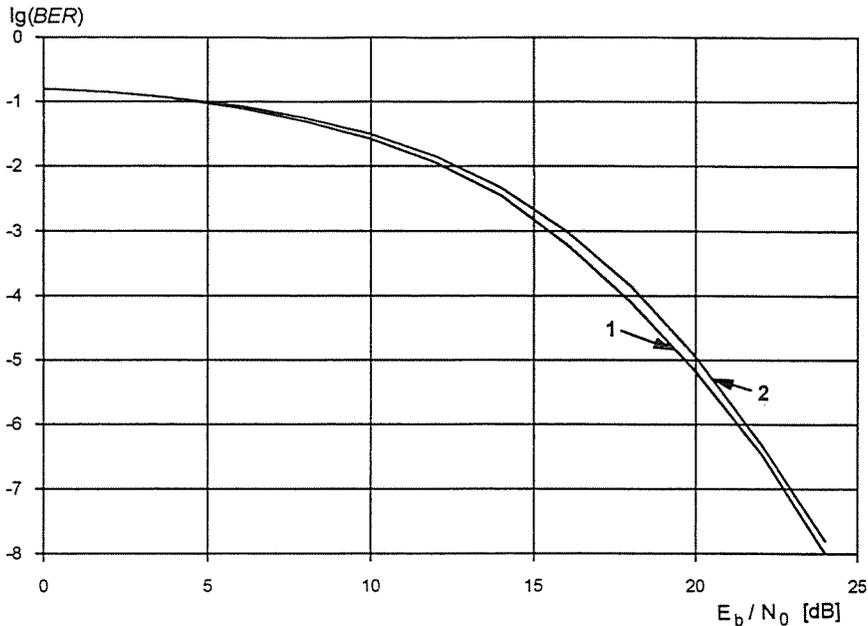
Fig. 8. Lower bound and upper bound of  $BER$  for the 64-QAM given in [11]. HPA is given in [12] with predistorter,  $BO_p = 2$  dB. 1: result of ASTRAS-QL for the purely linear system; 2: result of the simple procedure
