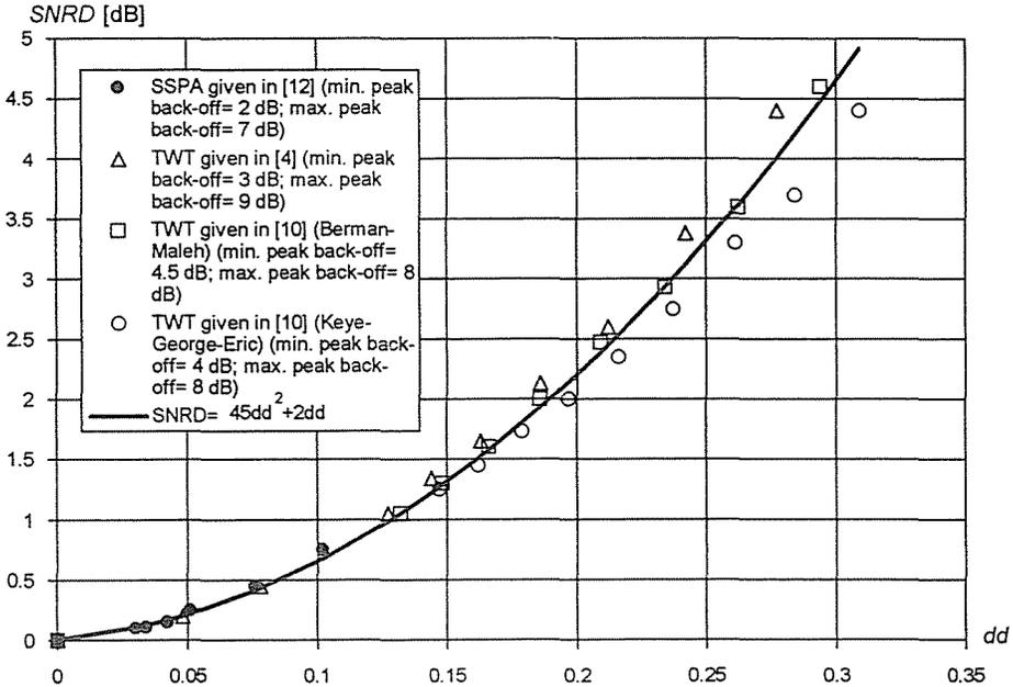
Fig. 3a. Relationship between  $SNRD$  (taken at  $BER = 10^{-6}$ ) and  $dd$
