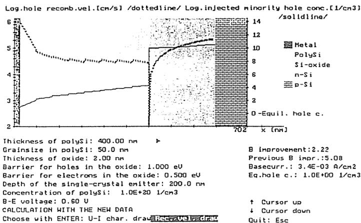
Fig. 4. ERV and concentration of minority holes from the metal contact to the E-B space-charge region. The major recombination takes place in the vicinity of oxide layer, which is also indicated by the discontinuity both in the ERV and the hole concentration curve. The same happens in the grain boundaries of the polysilicon, however, less significantly
