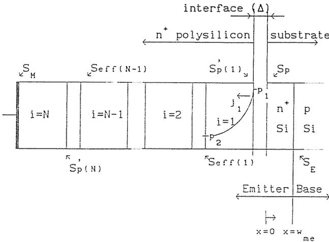
Fig. 2. One-dimensional box model of the polysilicon contact. The numbered boxes correspond to the grains, and between them there are the grain boundaries
