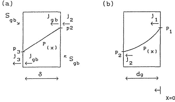
Fig. 1. Schematic diagram of the box model for the grain boundary (a), and for the grain (b)
