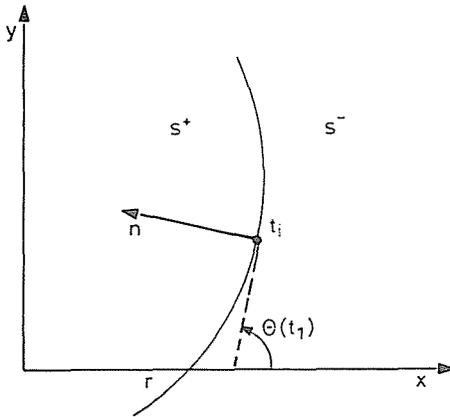
*Fig. 3.* The geometry for the electric field intensity on the boundary
