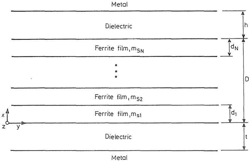
*Fig. 1.* Geometry of planar MSW waveguide
