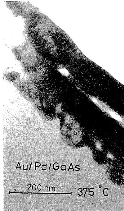
*Fig. 8.* Cross-sectional view of Au(50 nm)/Pd(50 nm)-GaAs sample heat treated at 375°C.
