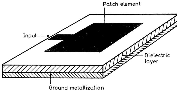
*Fig. 1.* A resonant element of Microstrip Antenna (MSA)
