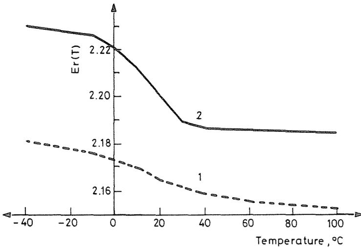
Fig. 9. Dielectric constant variation over temperature, calculated from measurement data
