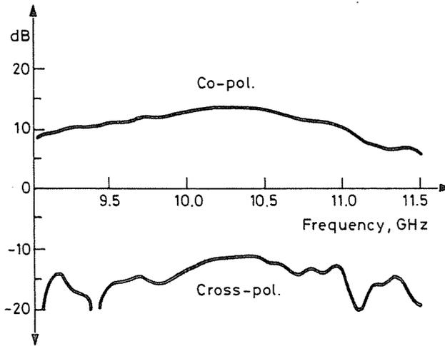
Fig. 11. Co- and cross-polarized gain of a two by two element MSA array
