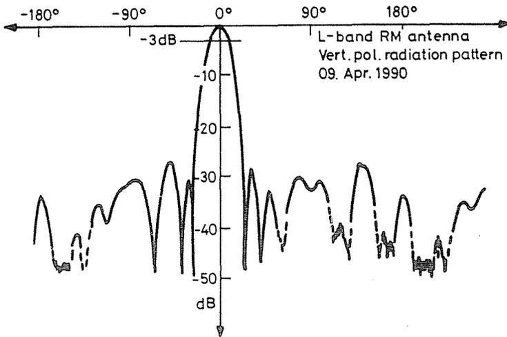
Fig. 5. Radiation pattern of MSA for microwave radiometer
