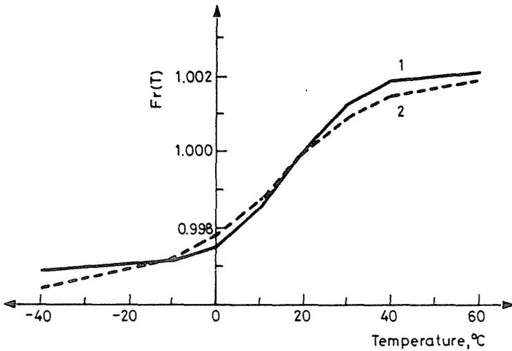
Fig. 8. Measured resonance frequency of MSA over temperature
