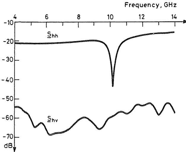
Fig. 10. Radar Cross Section of a single MSA element without feeding
