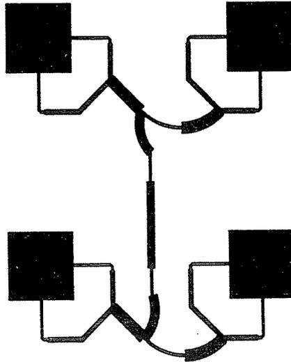
Fig. 3. Circularly polarized MSA
