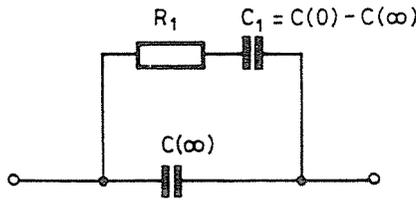
Fig. 2. The Debye model ( $\tau_D = R_1C_1$ )
