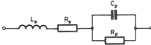
*Fig. 1.* The wide frequency range capacitor model
