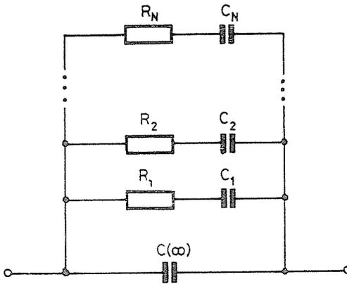
*Fig. 3.* Capacitor model with a distribution of relaxation times ( $\tau_i = R_i C_i$ ;  $k_d = \sum_{i=1}^N C_i / C(\infty)$ )
