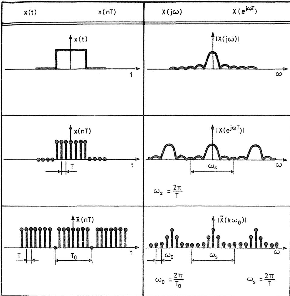
Fig. 2. An example for the connection between continuous- and discrete-time Fourier transform
