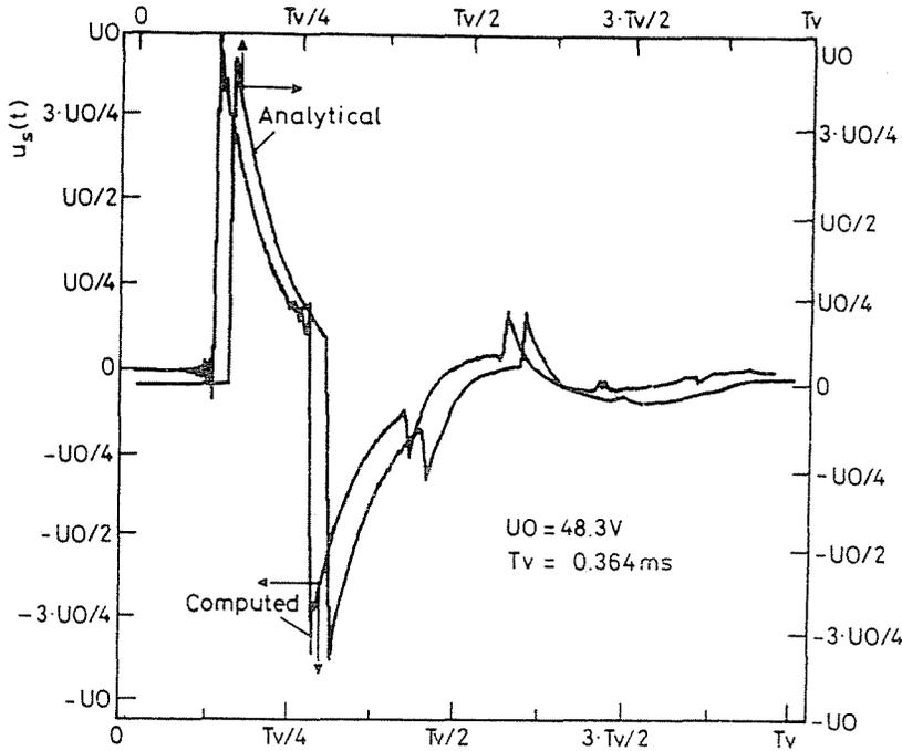
Fig. 5. The analytical and the computed voltage functions at the load of the transmission line in Fig. 3, if it is lossy but distortionless
