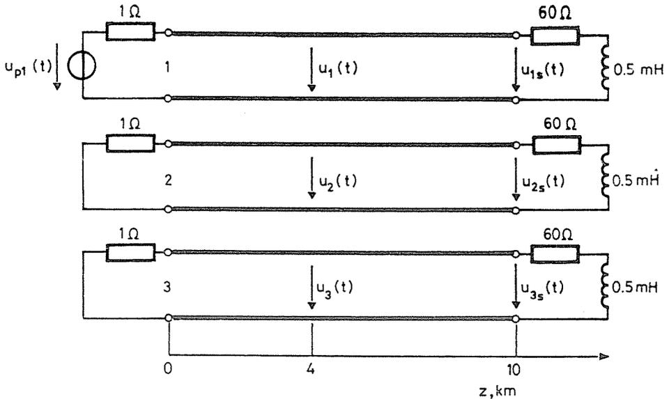
Fig. 6. The transmission line system discussed in Example 2
