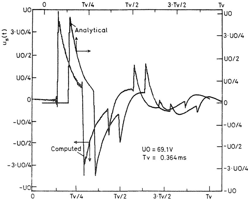
Fig. 4. The analytical and the computed voltage functions at the load of the transmission line shown in Fig. 3, if it is loss-free
