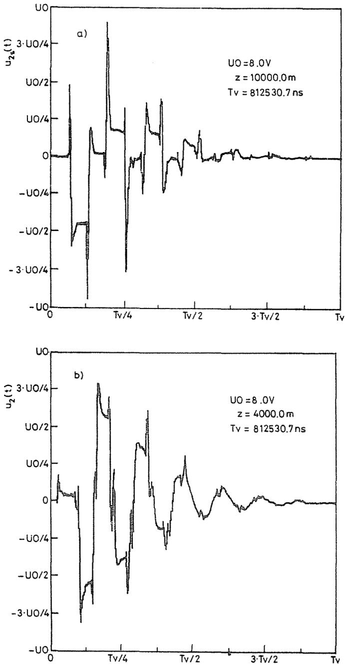
Fig. 9. The computed voltage functions of Line 2 (see Fig. 6)
