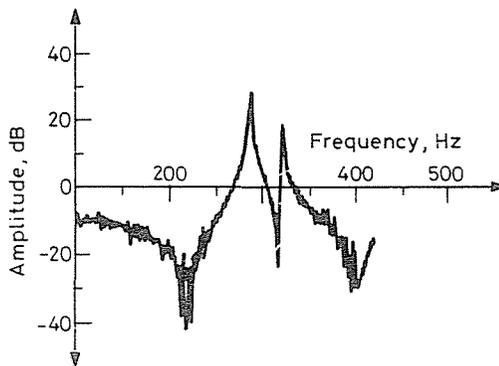
Fig. 4. Measured and estimated transfer function of a vibrating mechanical system
