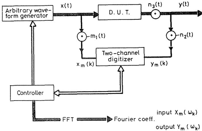
Fig. 1. Schematic presentation of the measurement system
