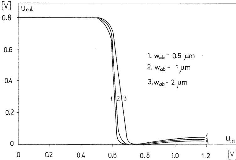
Fig. 8. Transfer characteristic dependence on the change of the active base thickness ( $w_{ab}$ )
