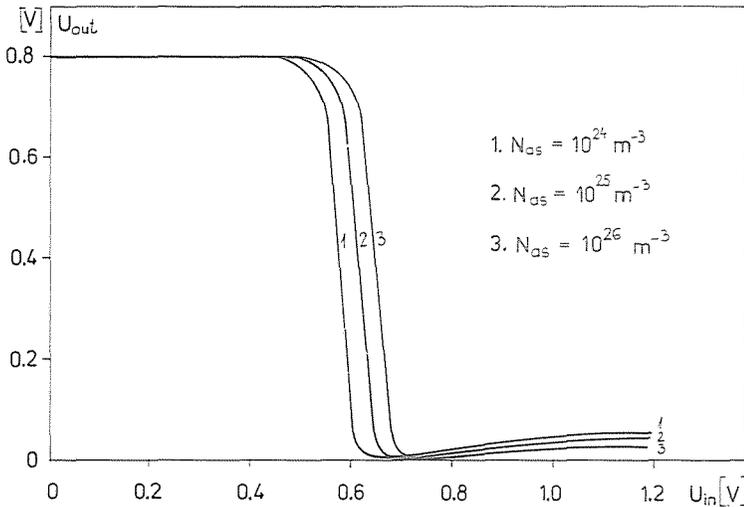
Fig. 6. Transfer characteristic dependence on the change of the base surface concentration ( $N_{as}$ )
