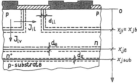
Fig. 3. Lateral pnp part of the I<sup>2</sup>L gate
