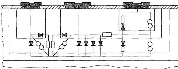
Fig. 1. Structure oriented model of the  $I^2L$  gate
