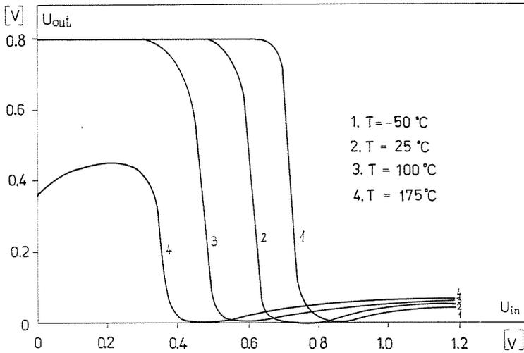
Fig. 9. Transfer characteristic dependence on the change of the temperature ( $T$ )
