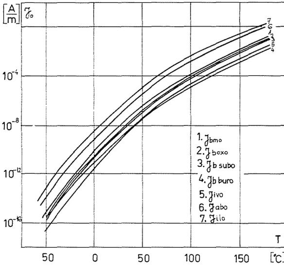
Fig. 5. Saturation currents ( $J_s$ ) dependence on temperature ( $T$ )
