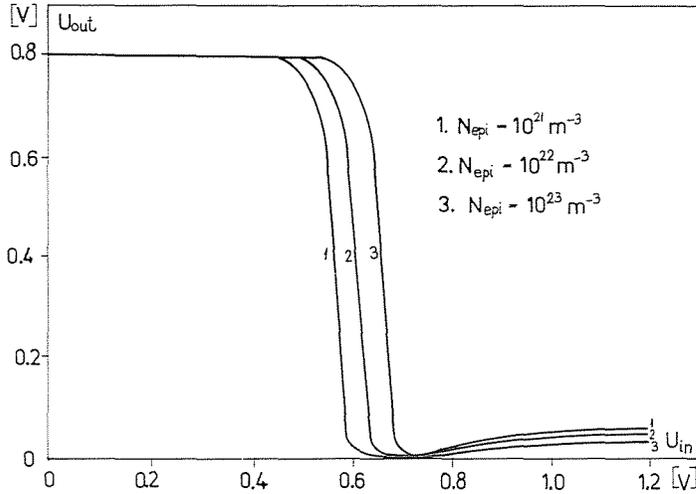
Fig. 7. Transfer characteristic dependence on the change of the epitaxial layer concentration ( $N_{epi}$ )
