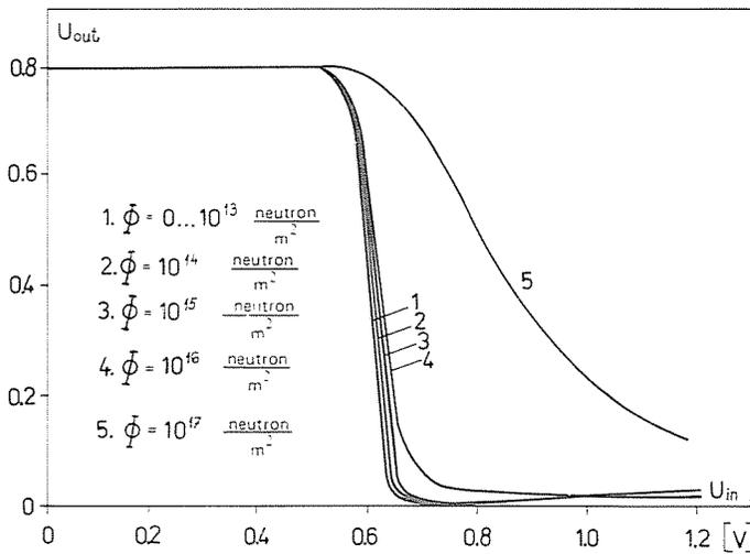
Fig. 10. Transfer characteristic dependence on the change of the neutron irradiation ( $\Phi$ )
