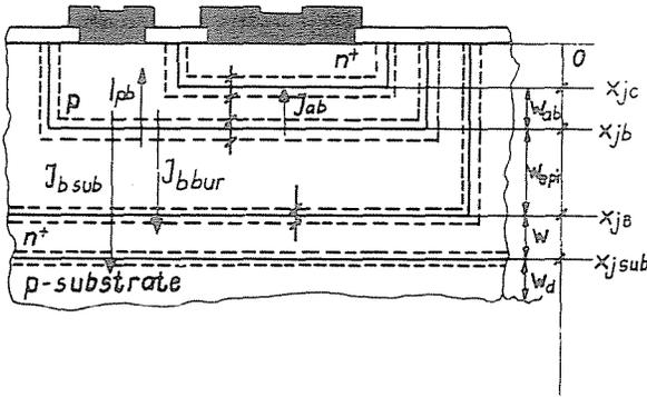
Fig. 4. Vertical npn part of the I<sup>2</sup>L gate
