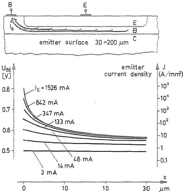
Fig. 6. Distribution of emitter-base voltage and emitter current density in a high-power planar transistor calculated with circuit analysis program
