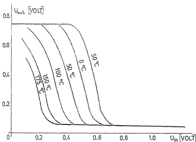
Fig. 9. Transfer characteristics of the  $I^2L$  element at different temperatures
