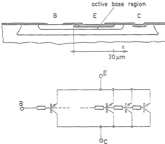
Fig. 5. Model of a bipolar transistor for examining the current crowding phenomenon
