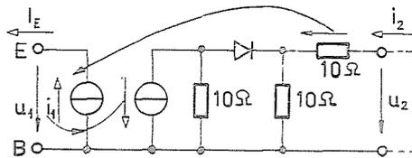
Fig. 3. Models of the junctions around the base region
