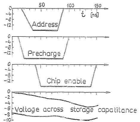
Fig. 12. Voltage drop on the capacitance of the 1103 dynamic storage cell at logical "0" and "1" level. The voltage level is evaluated at the 100 nsec time instant
