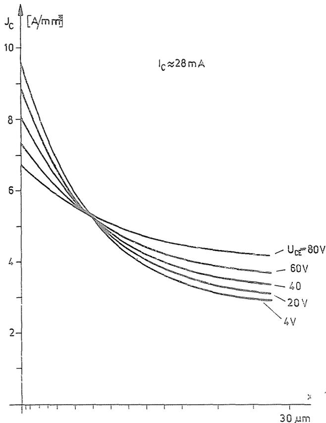
Fig. 7. Emitter current density distribution in the case of current crowding considering also the thermal coupling of the base lumps
