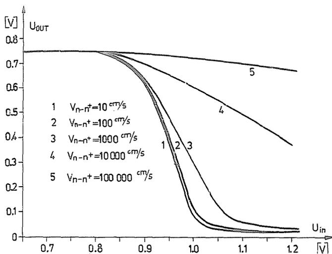
Fig. 10. Dependence of the  $I^2L$  transfer characteristics on the  $n-n^+$  (buried layer) recombination velocity
