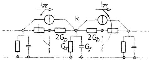
Fig. 2. Lumped model of the base region
