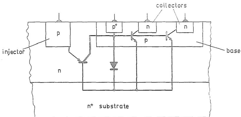
Fig. 8. Simple model of an  $I^2L$  element
