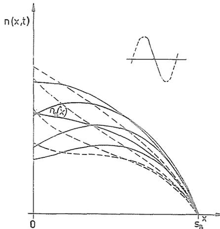
Fig. 4. Minority carrier distribution calculated using the regional approximation method based on Linvill's idea, with a sinusoidal excitation at different time instants
