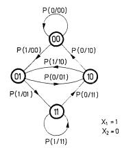
Fig. 3. State-diagram of a simple Markov-source
