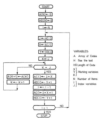
Fig. 7. Generating the coding scheme
