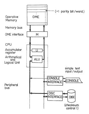
Fig. 10. Schematic model and data paths of minicomputers
