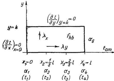
Fig. 2. A quarter of the winding disc as a space part under examination, with the conditions of calculation
