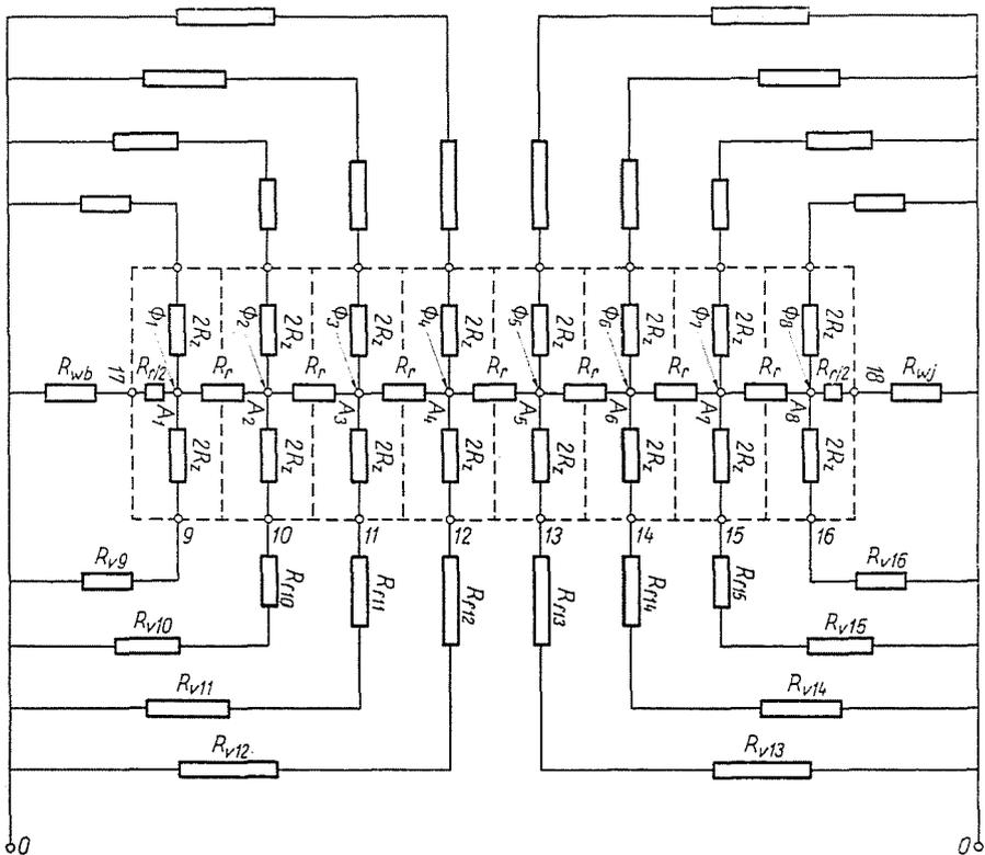
Fig. 3. Heat flux network model of a coil disc for steady state ( $\Phi$ : source heat fluxes)
