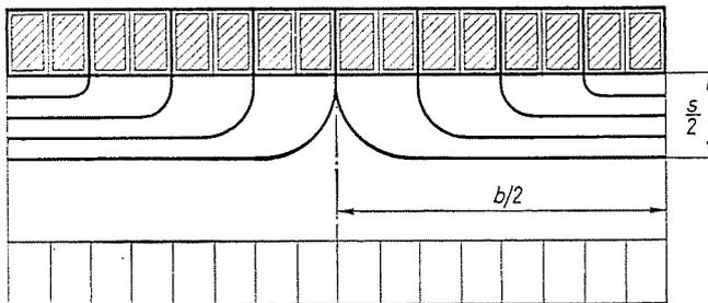
Fig. 1. Block scheme of the coil disc, paths of turbulent heat conduction ( $b$ : disc width,  $s$ : thickness of the horizontal oil duct)
