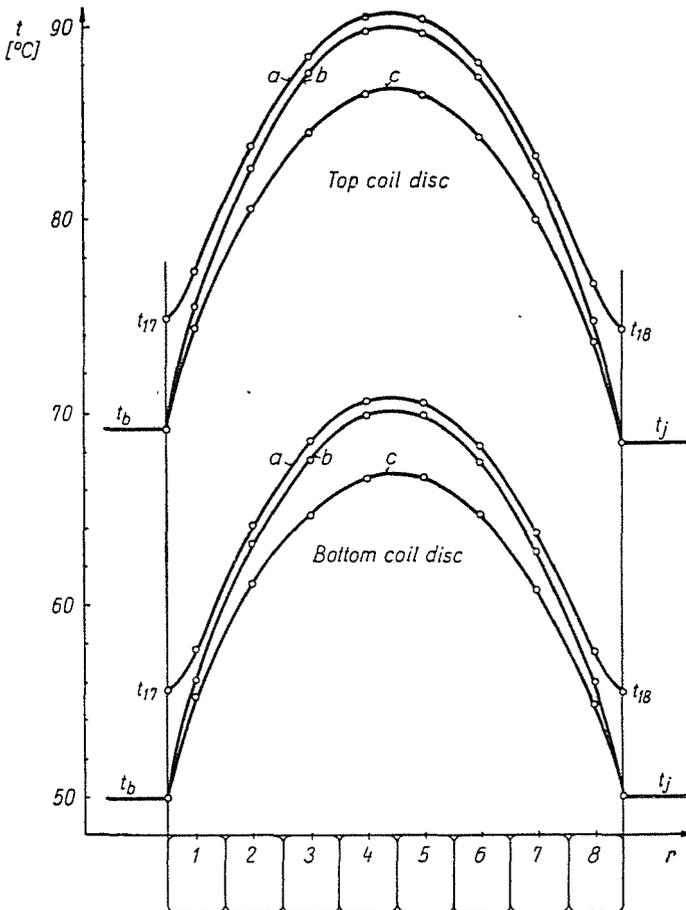
Fig. 6. Temperature distribution in the bottom and top coil discs of a coil column, based on the heat flux network model in Figs. 4 and 5. (a: temperature of the copper conductor; b: temperature of the outer surface of the paper insulation; c: mid oil temperature)
