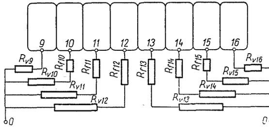
Fig. 2. Resistance network representing the mixed (turbulent) heat conduction of the horizontal oil duct
