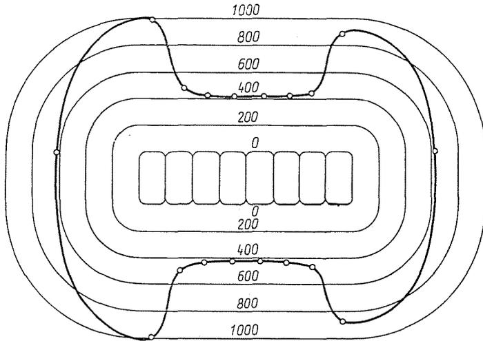
Fig. 7. Distribution of heat flux density on the surface of the hottest coil disc
