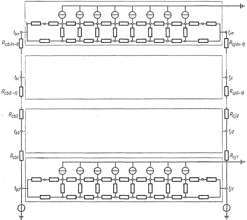
Fig. 5. Heat flux network model of a whole coil column
