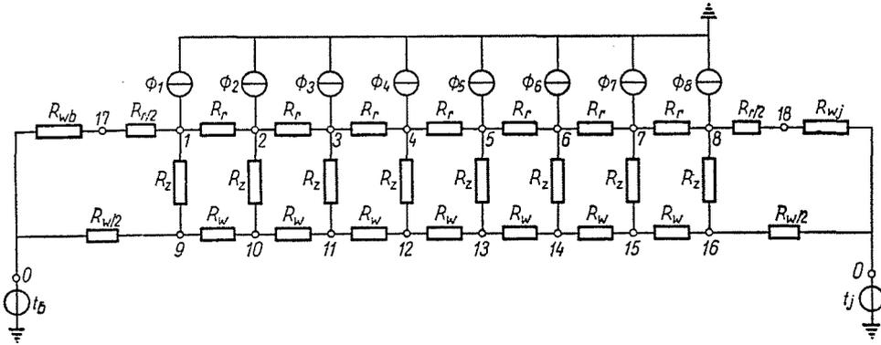
Fig. 4. Reduced heat flux network model of a coil disc for steady state
