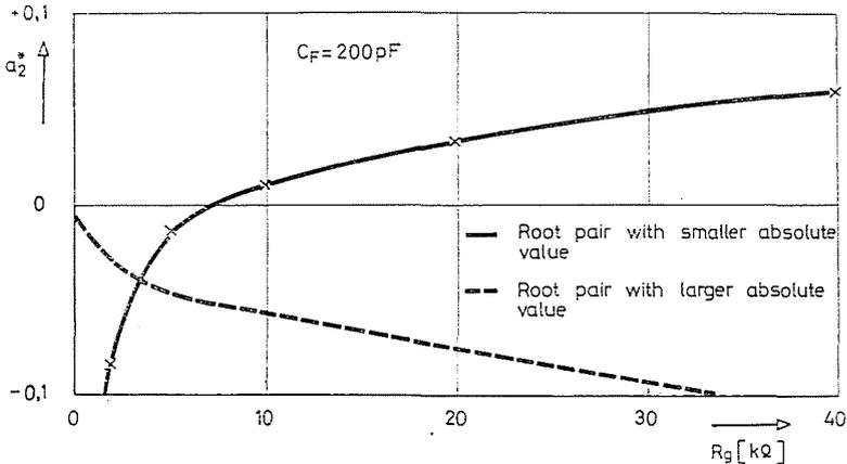
Fig. 13. Relative distances of two closed-loop pole-zero pairs of the amplifier type 748 with feedforward compensation, as a function of the generator resistance ( $C_F = 200 \text{ pF}$ )
