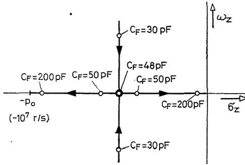
Fig. 10. Zero loci of the closed-loop transfer function of the amplifier type 748 with feed-forward compensation
