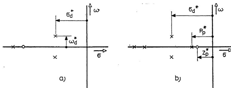
Fig. 3. A typical pole-zero configuration of the closed-loop transfer function of operational amplifiers
