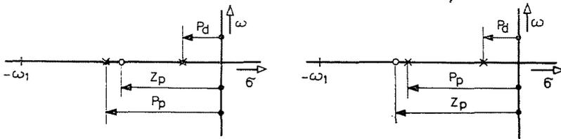
Fig. 4. Pole-zero configuration of the open-loop transfer function of operational amplifiers in the presence of a parasitic pole-zero pair
