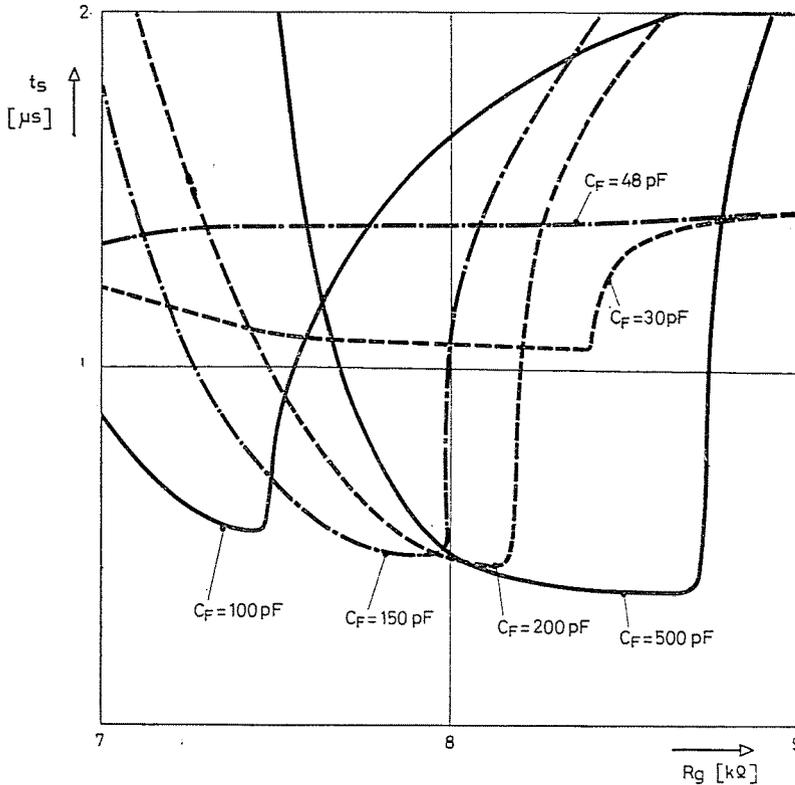
Fig. 14. Settling time of a unity gain inverting amplifier with the operational amplifier type 748 of feedforward compensation
