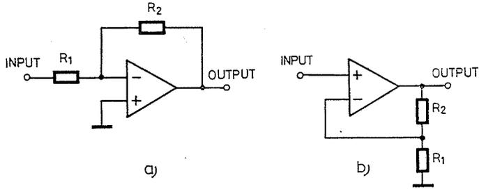
Fig. 1. Inverting (a) and noninverting (b) operational amplifiers
