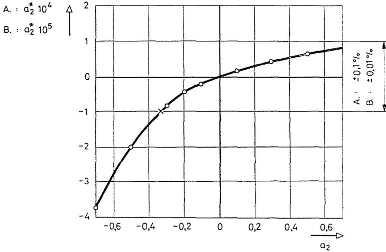
Fig. 6. Interrelation between the relative distances of the parasitic open-loop and closed-loop pole-zero pairs of feedforward operational amplifiers
