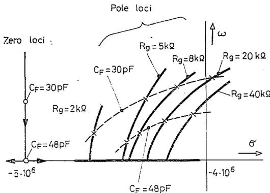
Fig. 12. Root loci of the closed-loop transfer function of the amplifier type 748 with feed-forward compensation. An enlarged detail
