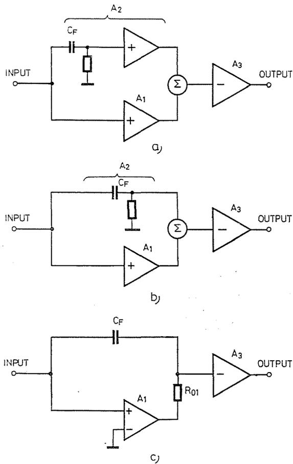
Fig. 2. Three main types of the application of feedforward
