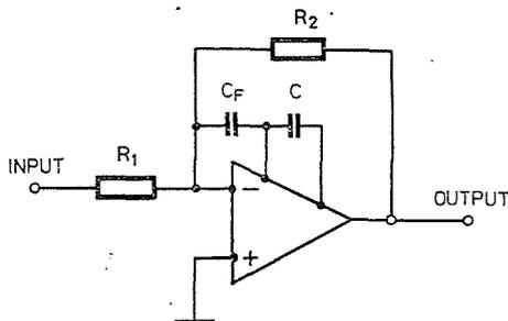
Fig. 8. Inverting amplifier with an integrated operational amplifier of feedforward compensation
