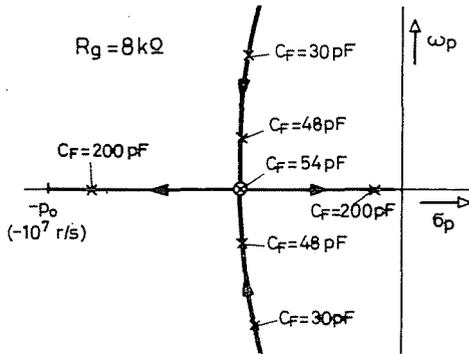
Fig. 11. Zero loci of the closed-loop transfer function of the amplifier type 748 with feed-forward compensation ( $R_g = 8$  kohm)
