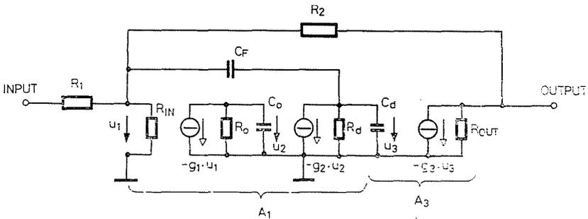
Fig. 9. Linear model of the circuit shown in Fig. 8
