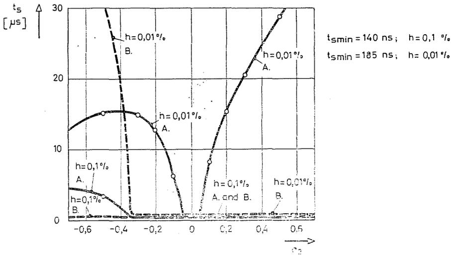
Fig. 7. Settling time of feedforward operational amplifiers as a function of the distance of the open-loop pole-zero pair
