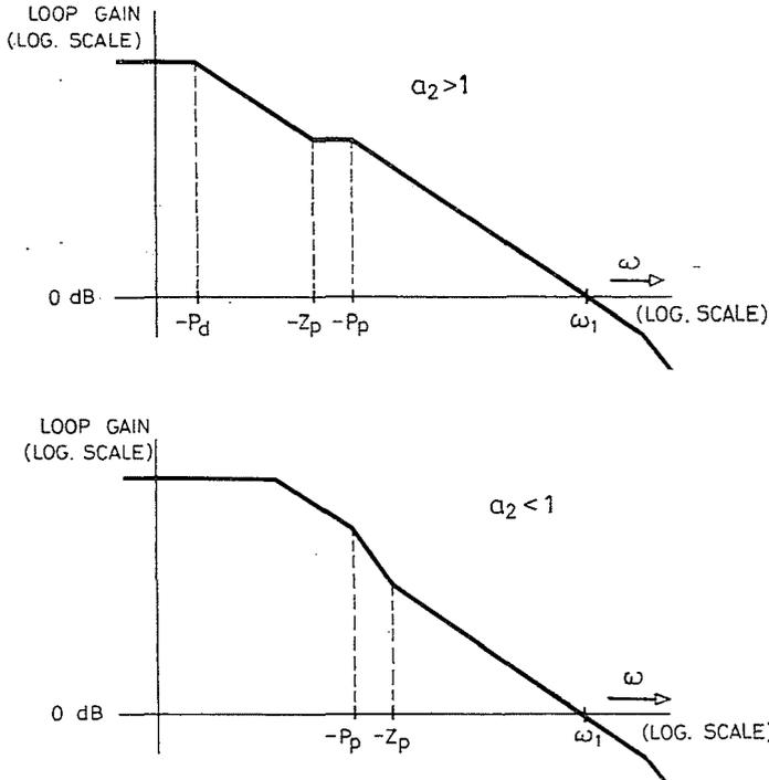
Fig. 5. Absolute value of the loop gain of operational amplifiers as a function of frequency, in the presence of a parasitic pole-zero pair
