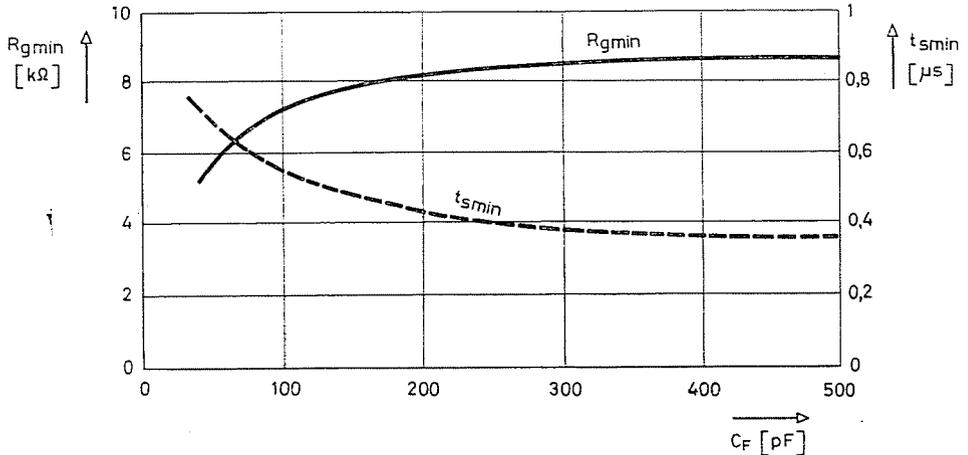
Fig. 15. Optimum generator resistance and minimum settling time vs. feedforward capacitance  $C_F$
