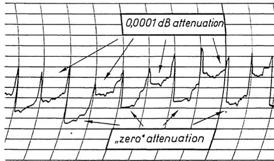
Fig. 4. Resolution of the A.F. substitution system for attenuation measurement
