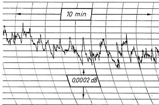
Fig. 5. Short-time stability of the A.F. substitution system for attenuation measurement
