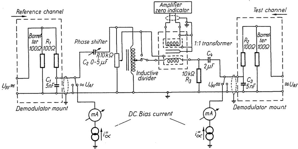
Fig. 2. Diagram of A.F. circuitry of audio substitution attenuation measuring set with R.F. barretter demodulators
