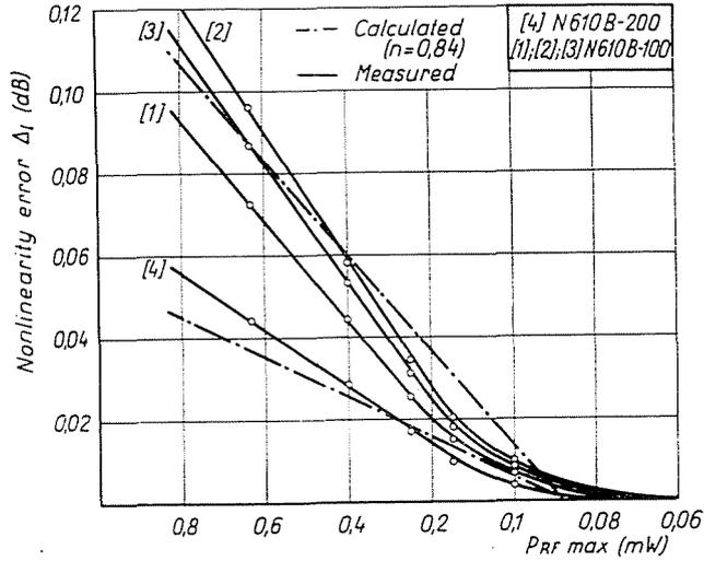
Fig. 3. Comparison of calculated and measured nonlinearity error for barretters
