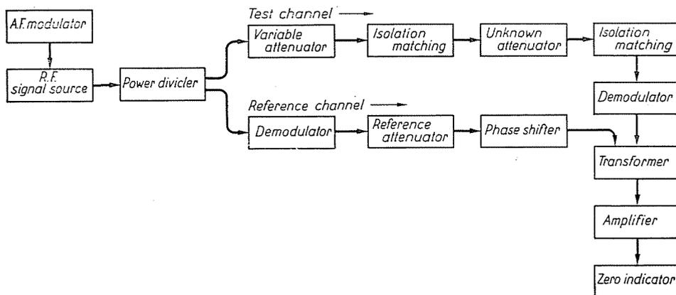
Fig. 1. Double channel audio modulation substitution system for attenuation measurement
