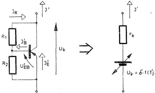
Fig. 5. Compensating transistor circuit and its equivalent circuit
