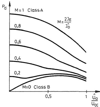
Fig. 10 Variation of the dissipated power at different operating points vs. output level (sinusoidal signal)
