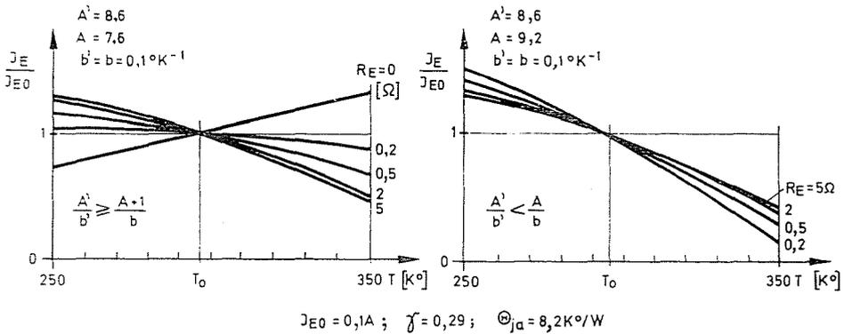
Fig. 7. Characteristic temperature-dependence of the current of the power transistors for various ratios of parameters  $A$  to  $A'$
