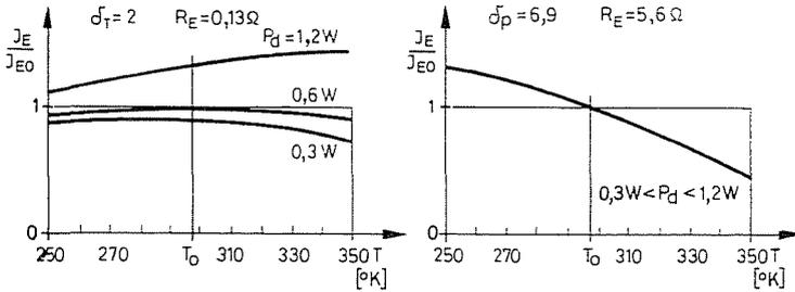
Fig. 11. Dependence of the operating point current on ambient temperature and dissipation
