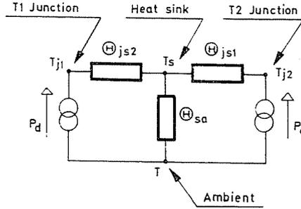
Fig. 4. Simplified thermal equivalent circuit of the power transistors
