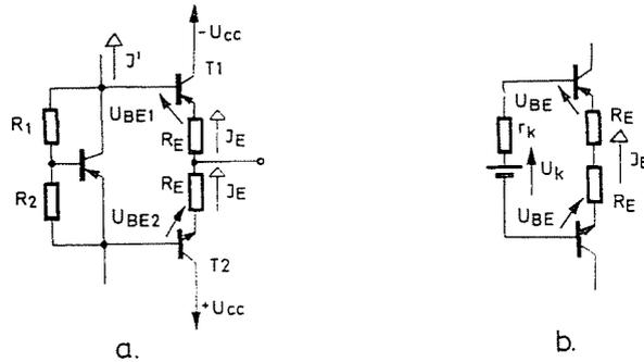
Fig. 6. Biasing of the power transistors (a), and simplified equivalent circuit (b)
