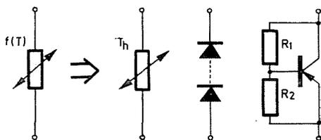
Fig. 3. Circuit elements for biasing the temperature-dependent operating point: a) thermistor, b) diodes biased in forward direction, c) transistor circuit.
