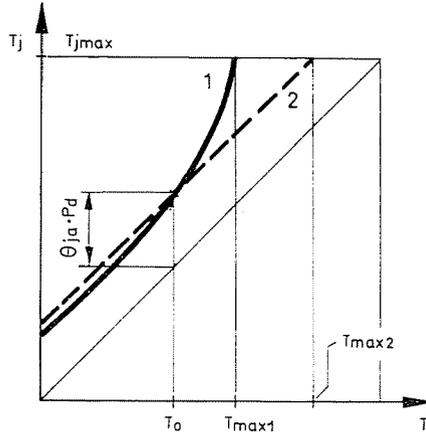
Fig. 1. Change of the junction temperature vs. ambient temperature, for temperature-dependent  $I_E$  (1) and constant  $I_E$  (2)
