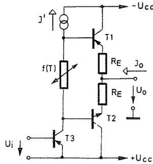
Fig. 2. Circuit diagram of a complementary symmetry power amplifier
