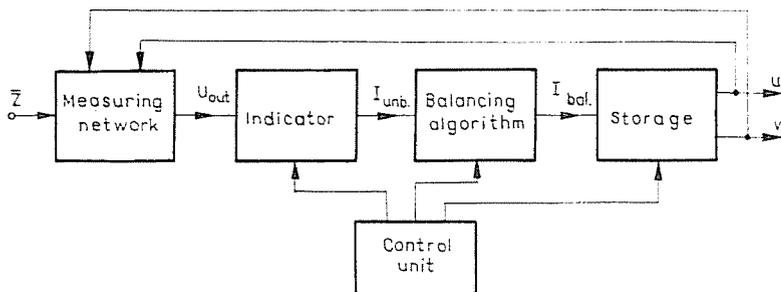
Fig. 1. The general scheme of precision balanced measurements
