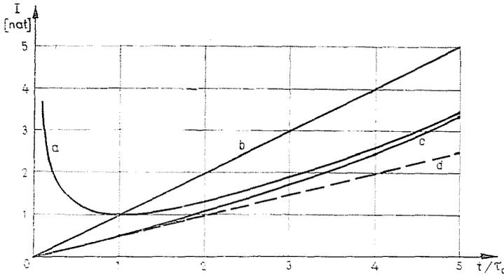
Fig. 9. Information content of measurement vs. holding time. a) uncertainty of time constant; b) noise of indicator; c) resultant transformation; d) information content of practical measurement
