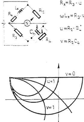
Fig. 2. Balancing trajectory of Maxwell—Wien bridge
