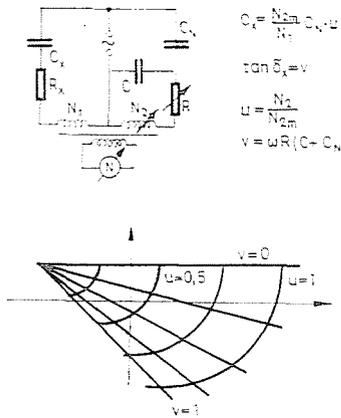
Fig. 3. Balancing trajectory of ideal current comparator faradmeter network
