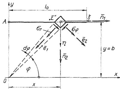
Fig. 5. Stresses arising in point  $E$  of the longitudinal axis of a strain gauge of length  $l_0$
