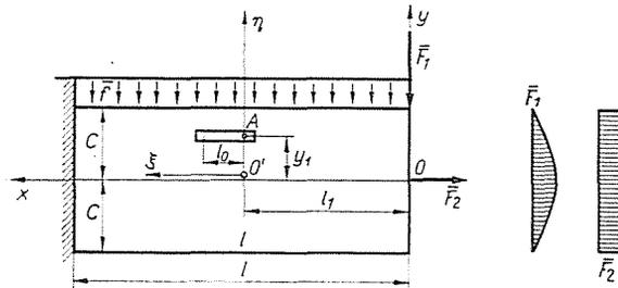
Fig. 2. Cantilever beam with a strain gauge of length  $l_0$  at point  $A$
