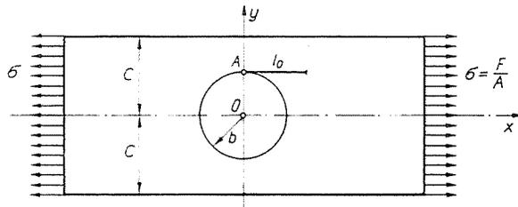
Fig. 4. Tensile plate with circular hole and strain gauge at point  $A$
