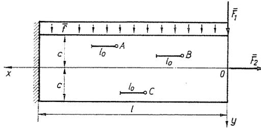
Fig. 3. Cantilever beam with strain gauges at points  $A$ ,  $B$  and  $C$
