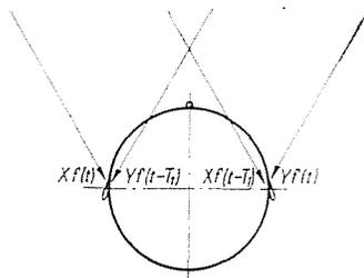
Fig. 13. The paths of the sounds reaching the ear in case of two channel stereo sound reproduction
