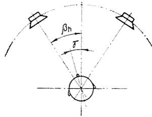
Fig. 10. The observer positioned at an angle  $\gamma$  to the symmetry plane of the sound reproduction system
