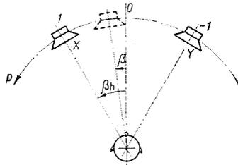
Fig. 1. Stereo sound reproduction system using two loudspeakers
