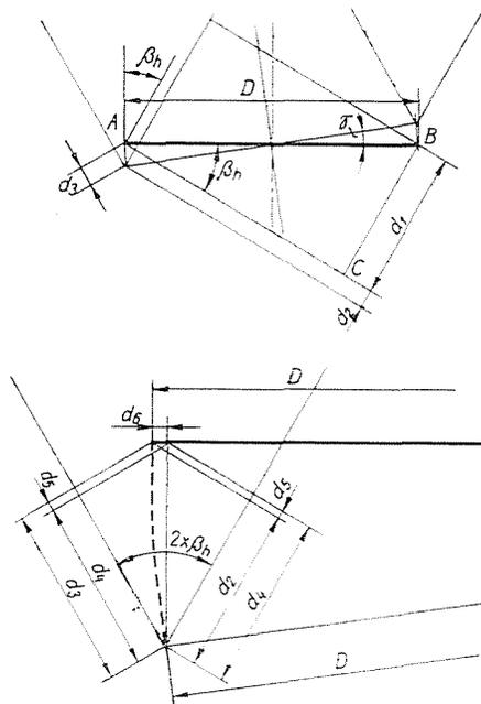
Fig. 14. For the calculation of the sound pressure of the left ear in case the head forms an angle  $\gamma$  with the symmetry axis of the system
