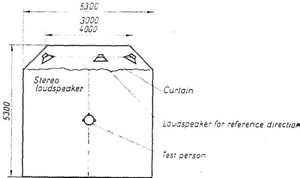
Fig. 6. The positioning of the two loudspeakers and the observer for the determination of the direction of the virtual sound source
