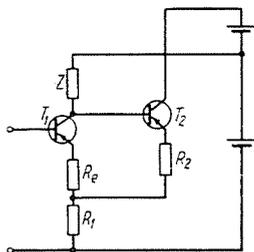
Fig. 3. Transistorized equivalent of the circuit of Fig. 1
