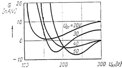
Fig. 7. Output conductance of the circuit of Fig. 5 plotted against  $U_{a1}$
