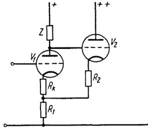
Fig. 1. Basic circuit to realize infinite inner resistance
