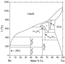
Fig. 3. Sn-Cu phase diagram
