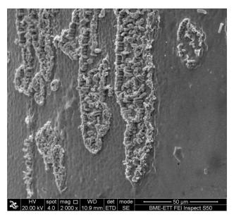
Fig. 1. Whisker development on the corrosion spots in the 96Sn4Cu samples at 1200 hours
