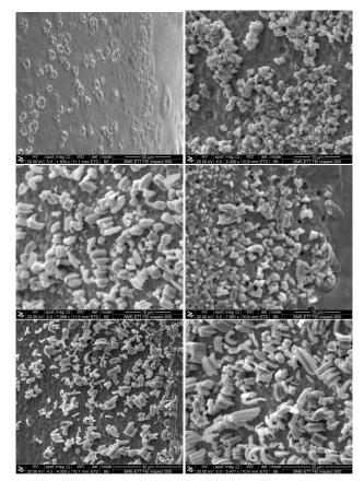
**Fig. 2.** Whiskering on the corrosion spots at 2000 hours on samples with the following percentage of copper: a. 0%, b. 1%, c. 2%, d. 3%, e. 4%, f. 5%.
