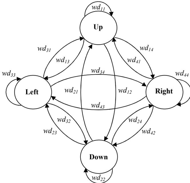
**Fig. 2.** Four state Markov chain to model the direction of rain cell translation
