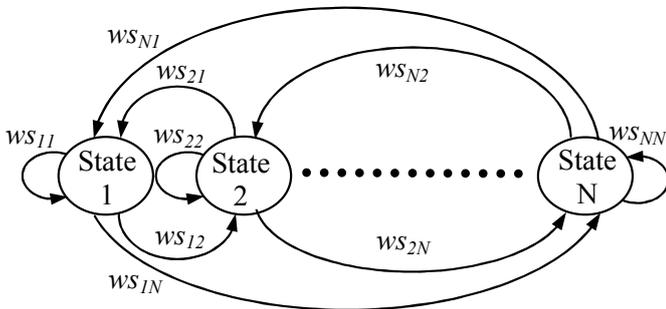
Fig. 5. Markov model of the wind speed
