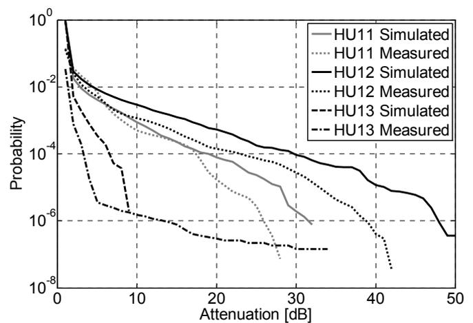
**Fig. 10.** Simulated and measured rain attenuation CCDFs
