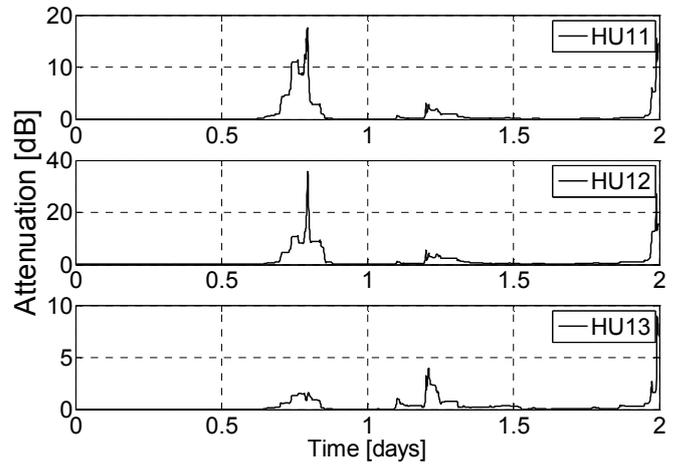
Fig. 8. Simulated rain attenuation time series; translation of one rain cell over the link area
