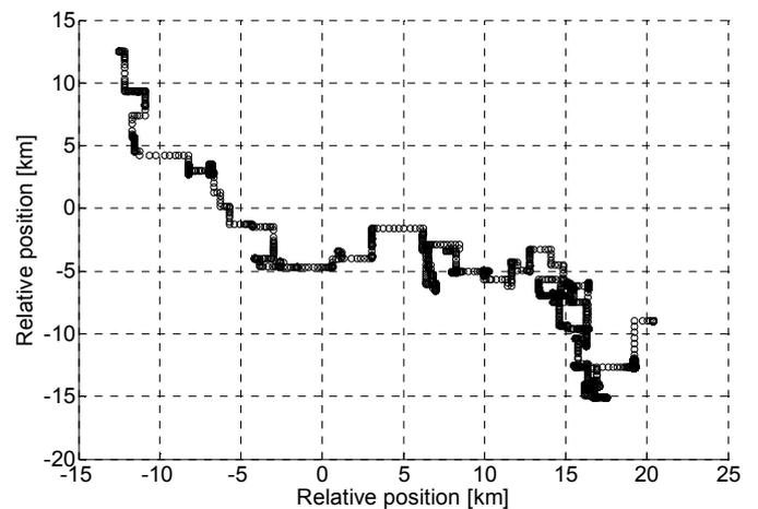
Fig. 6. Realization of a rain cell movement on the scene according to the Markov chain model (duration of 48 hours)
