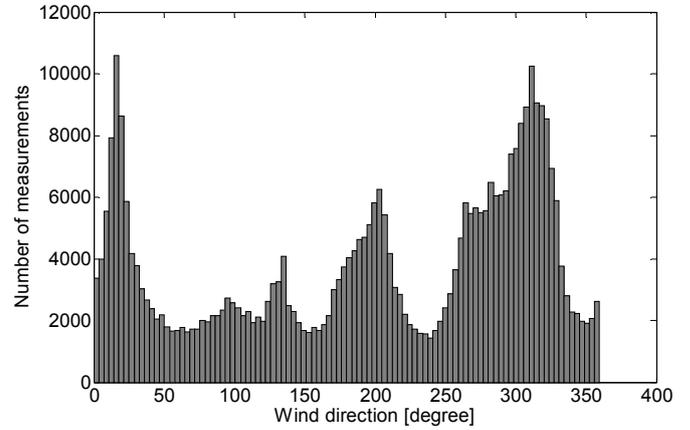
**Fig. 3.** Measured wind direction statistics. The angle is given in degrees; measured clockwise from North.
