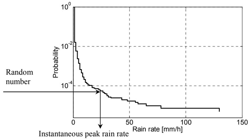
and 1 is generated to select the actual peak rainfall rate probability. The corresponding rain intensity can be read from the vertical axis of the CCDF and this value will be applied as the peak rain rate in the EXCELL model. The process is graphed in Fig. 9.
