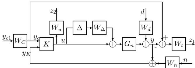
**Fig. 5.** The  $\Delta$ - $P$ - $K$  structure.  $G_n$  is the nominal plant,  $y_c$  the yaw-rate reference,  $y_{c1}$  the normalized yaw-rate reference,  $n$  denotes sensor noise,  $z_1, z_2$  performance signals,  $W_C, W_u, W_t, W_\Delta, W_d$  and  $W_n$  are weighting functions,  $K$  is the controller
