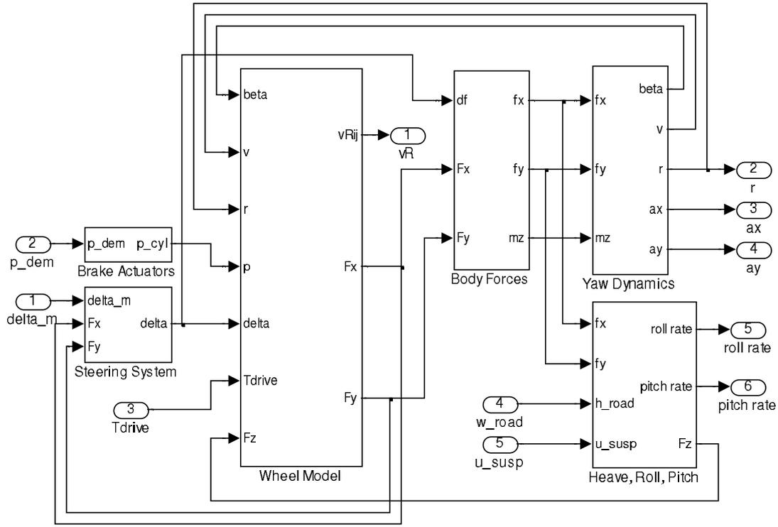
**Fig. 3.** Simulink block structure of the vehicle model. The input signals to the model are the followings: brake pressures to the four wheels ( $P_{dem}$ , zero for the rear wheels), driver torque to the steering wheel ( $T_{drive}=0$ ), driving
