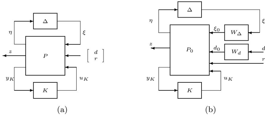
**Fig. 1.** (a)  $\Delta$ - $P$ - $K$ : the closed loop uncertain system in robust control. The unmodeled dynamics  $\Delta$  (block-diagonal) and the disturbance/noise  $d$  represent the model uncertainty,  $r$  stands for known signals (e.g. reference),  $z$  for error
