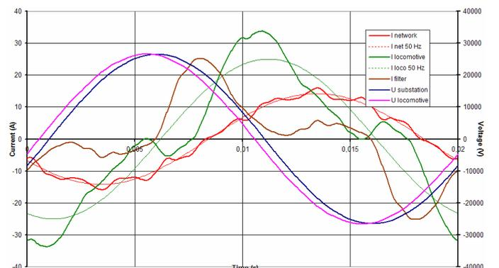
Fig. 17. Time functions with hybrid filtering (with 600 kvar reactive power)
