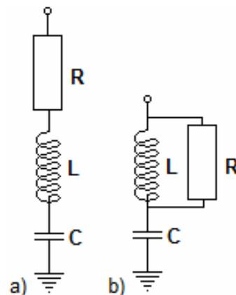
Fig. 19. Basic types of passive filters
