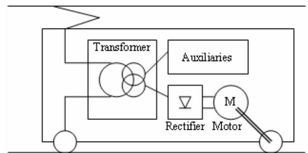
**Fig. 2.** Simplified block diagram of the Hungarian locomotives
