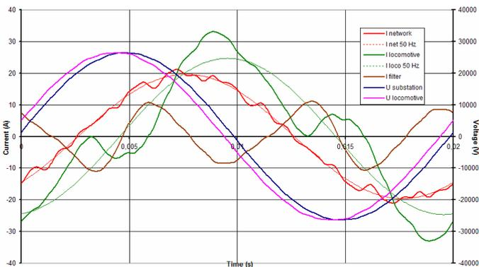
Fig. 13. Time functions with active filtering (ideal 21<sup>st</sup>-23<sup>rd</sup> filter included)
