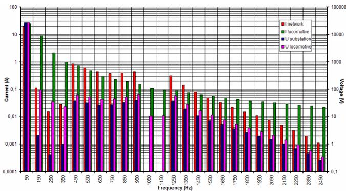
Fig. 12. Spectrums with active filtering (ideal 21<sup>st</sup>-23<sup>rd</sup> filter included)
