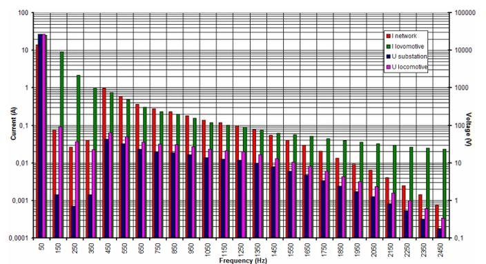
Fig. 16. Spectrums with hybrid filtering (with 600 kvar reactive power)
