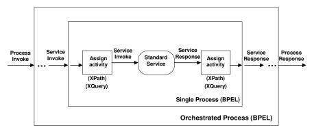
Fig. 4. Execution of a process request at proposal BPEL
