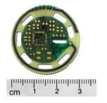
Fig. 13. Final size of the oximeter PWB
