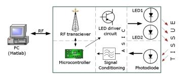
**Fig. 9.** Block diagram of the  $6^{th}$  generation device
