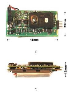
Fig. 8. a) top and b) side view of the previous oximeter
