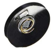
Fig. 6. Possible sensor head solution using a gold plated spiral shaped needle
