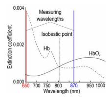
**Fig. 1.** Absorption spectrum of hemoglobin
