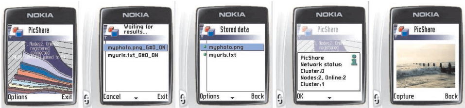
Fig. 7. NDS emulator: main screen & network events, query, content handling, net status, image capture
