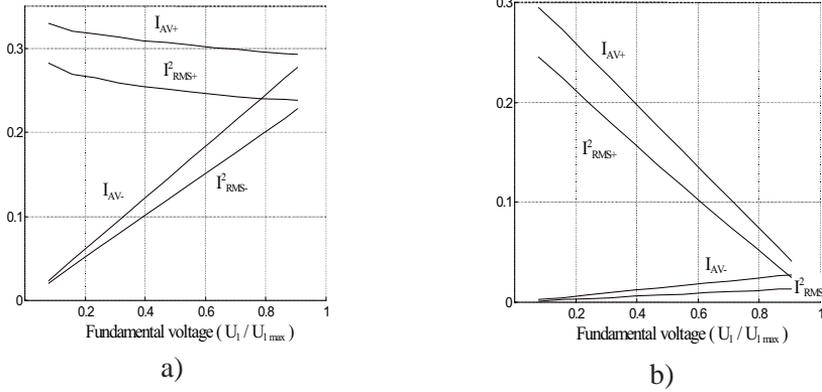
Fig. 8. Average current and square of rms current values of transistors (a) and diodes (b) of the positive (+) and negative (-) sides of the inverter bridge
