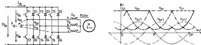
Fig. 1. Configuration of the inverter (a) and phase reference waves (b)
