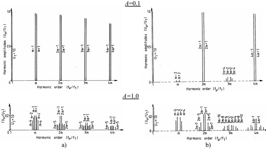
Fig. 5. Voltage spectra of two-phase (a) and three-phase PWMs (space vector method) (b) for  $A = 0.1$  and  $A = 1.0$
