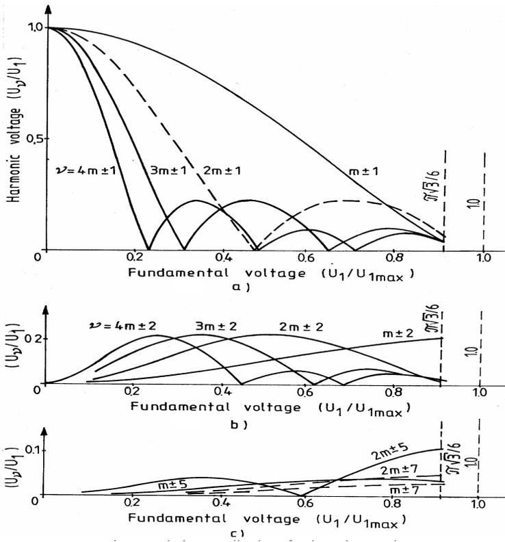
Fig. 4. Relative amplitudes of voltage harmonics
