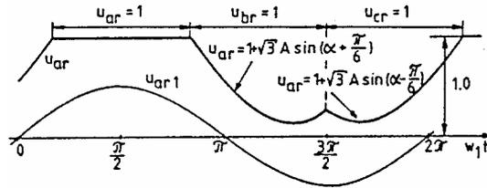
Fig. 2. The *a* phase reference wave and its fundamental component
