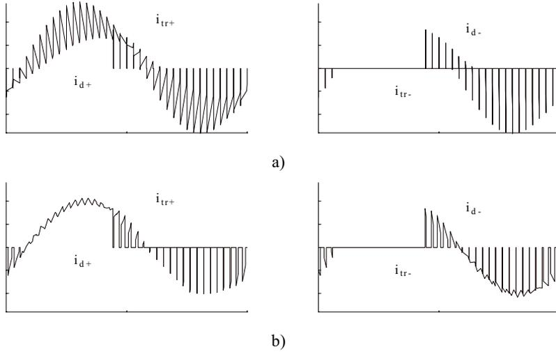
Fig. 7. Transistor and diode currents vs time for  $m = 36$  a)  $A = 0.1$  b)  $A = 2/\sqrt{3}$
