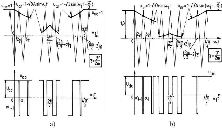
Fig. 3. Modulation processes for two-phase PWM with  $120^\circ$  and different initial phase angle of the carrier wave
