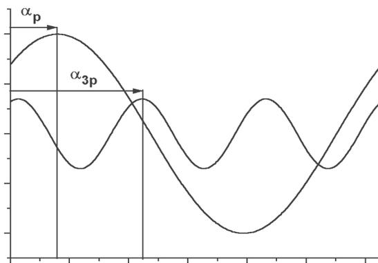
Fig. 1. The  $p$ - and the  $3p$ - harmonics of a total MMF
