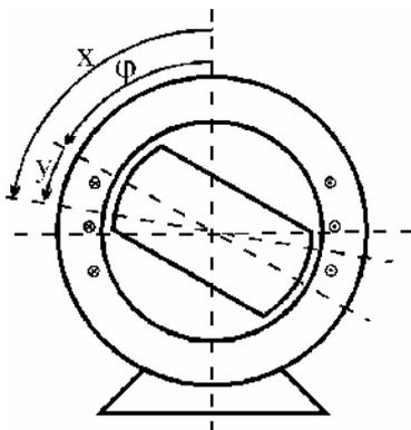
Fig. 2. An elementary one-phase converter
