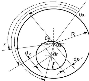
Fig. 3. Explanation of eccentricities: static, dynamic and mixed
