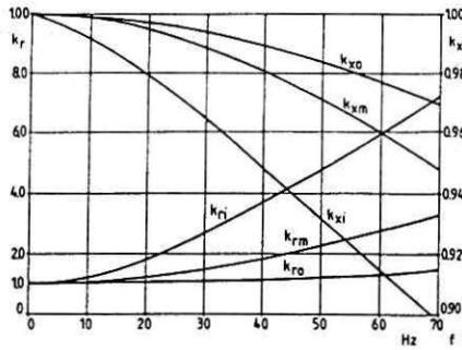
Fig. 8. Resistance and inductance skin factors of outer and inner bar
