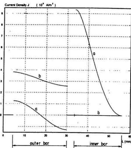
Fig. 3. Current density distribution along the symmetry axis ( $f = 50$  Hz). Instantaneous value at phase  $0^\circ$  is shown. a.)  $I_i = 1000$  A(peak)/ $0^\circ$ ,  $I_o = 0$ ; b.)  $I_i = 0$ ,  $I_o = 1000$  A(peak)/ $0^\circ$
