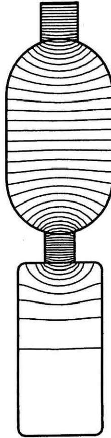
Fig. 2. Field lines at phase 0° if  $I_i = 1000 \text{ A(peak)}/0^\circ$ ,  $I_o = 0$  and  $f = 50 \text{ Hz}$ . Each flux tube contains 0.1 mWb/m.
