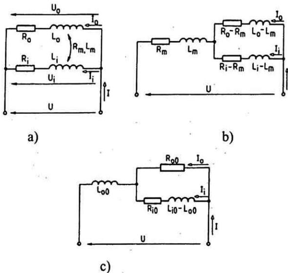
Fig. 7. Complete (a./) and modified complete (b./) equivalent circuits that include mutual impedance. Approximate equivalent circuit (c./). Values are unreferrred to stator.
