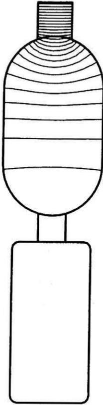
Fig. 4. Field lines at phase  $0^\circ$  if  $I_i = 0$ ,  $I_o = 1000$  A(peak)/ $0^\circ$  and  $f = 50$  Hz. Each flux tube contains  $0.1$  mWb/m.
