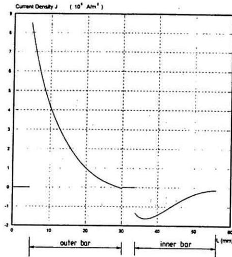
Fig. 6. Current density distribution along the symmetry axis ( $f = 50$  Hz). Instantaneous value at phase  $0^\circ$  if  $U_i = U_o = U = 0.1$  V/m(peak)/ $0^\circ$  is shown.
