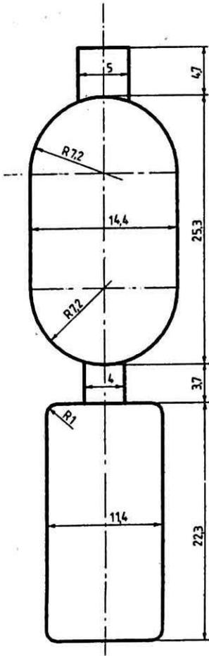
Fig. 1. Outline of rotor slot, outer and inner bar. All dimensions are in millimetres.
