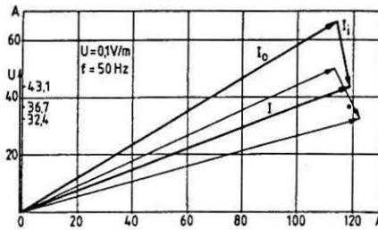
Fig. 9. Current phasors calculated from the correct and the approximate equivalent circuit
