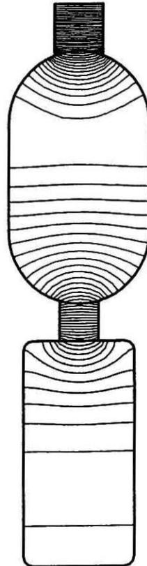
Fig. 5. Field lines at phase  $0^\circ$  if  $U_i = U_o = U = 0.1$  V/m(peak)/ $0^\circ$  and  $f = 50$  Hz. Each flux tube contains  $2\mu$ Wb/m.
