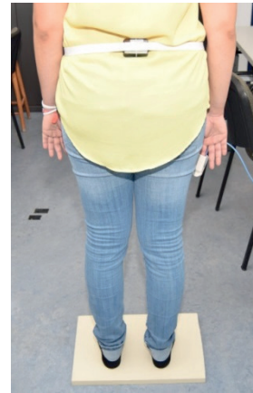
Fig. 2 Tested person standing on the floor. The PPG sensor was placed on the right index finger, and x-IMU was fixed to her back.
