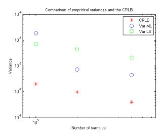
Fig. 1 Comparison of CRLBs of amplitude estimators
