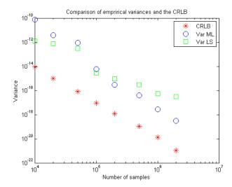
Fig. 3 Empirical variance of frequency estimators and the CRLB (simulated measurements)
