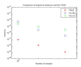
Fig. 5 Empirical variance of frequency estimators and the CRLB (real measurements)
