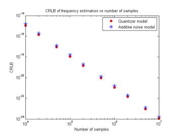
Fig. 2 Comparison of CRLBs of frequency estimators
