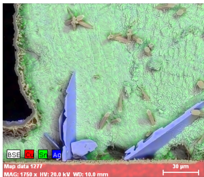
Fig. 3 Scanning electron microscope micrograph about a lead-free solder joint after the application of electrochemical etching.
