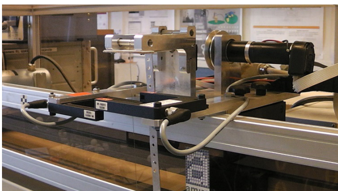
Fig. 11 Experimental crane system for the study of underactuated mechanisms
